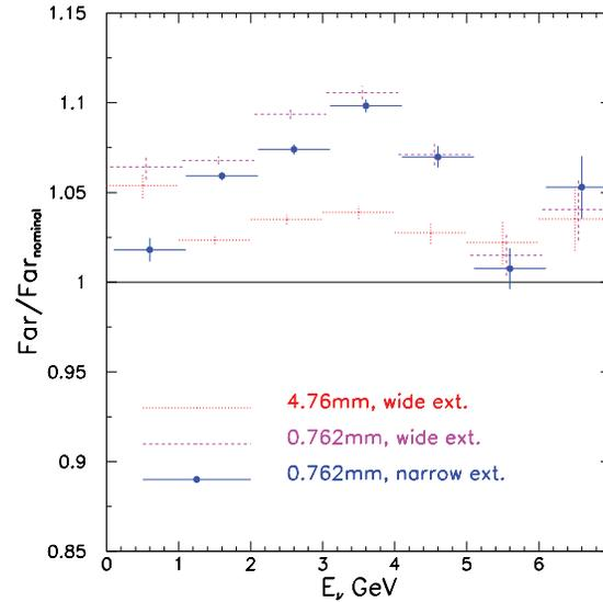
10% Increase in rate possible with extended pipe and thin window
