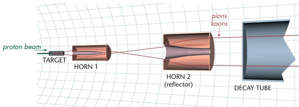
**Figure 7:** The production of pions and kaons (parents of the neutrinos), focussed in the direction of the Gran Sasso by two magnetic horns
