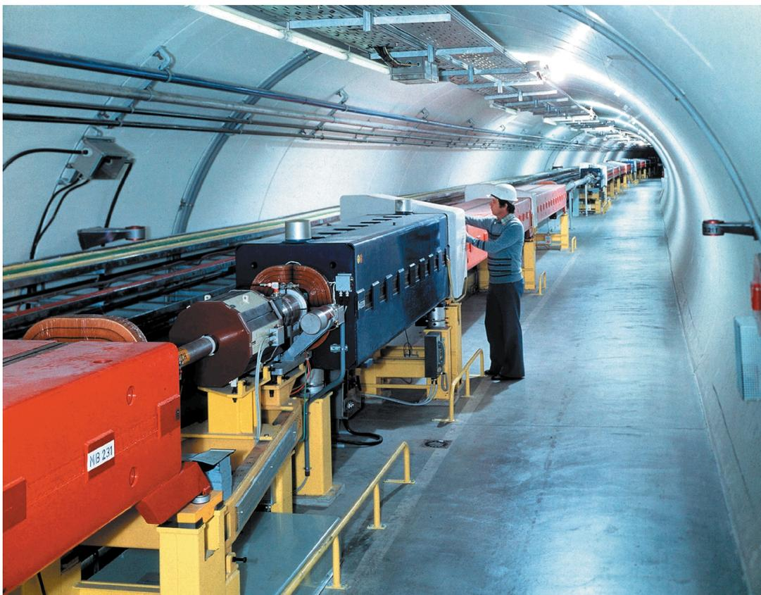
**Figure 9:** Dipoles (red) and quadrupoles (blue) in SPS tunnel
