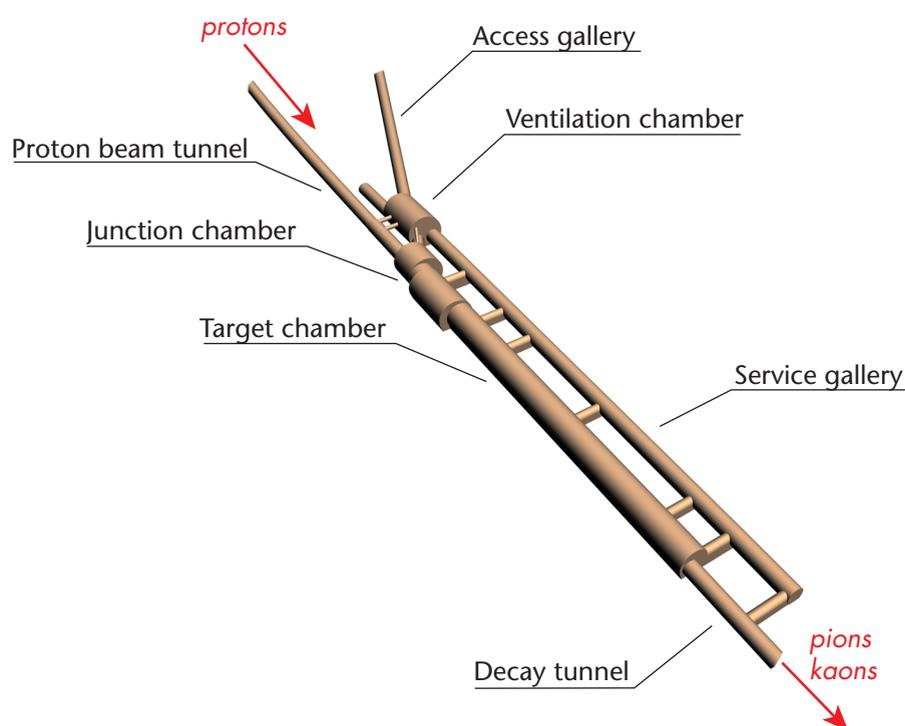
**Figure 13:** The target chamber and its annexes
