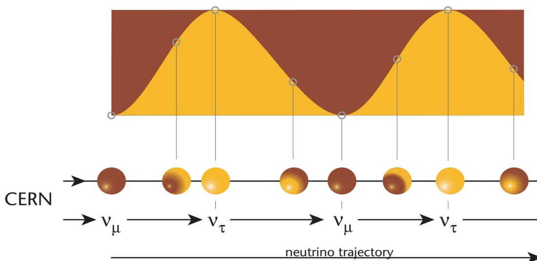
**Figure 2:** Illustration of  $\nu_\mu - \nu_\tau$  oscillations (a pure  $\nu_\tau$  beam is produced at CERN and directed towards Gran Sasso)
