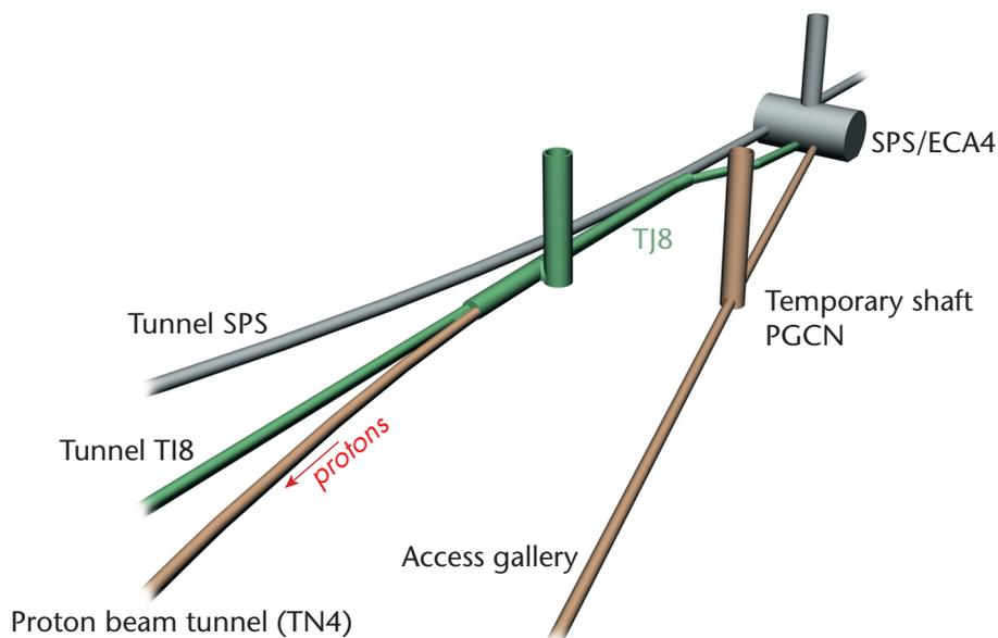
Figure 12: Underground work-sites at Point BA4 of the SPS. Tunnel T18, under construction, will connect the SPS to the LHC.
