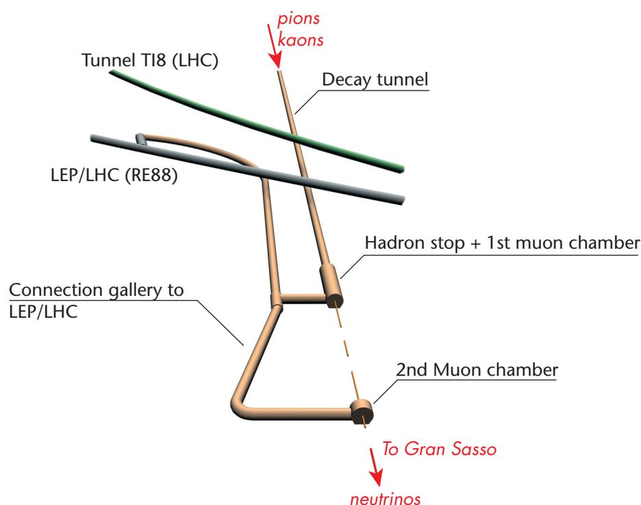
**Figure 14:** The hadron stop chamber and muon detection chambers and the connecting passages to the LEP/LHC
