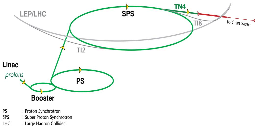
**Figure 8:** The CERN proton accelerators used for the CNGS
