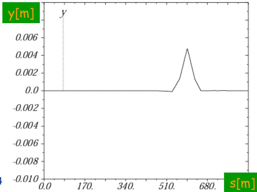
Vertical bump after correction along beam line
