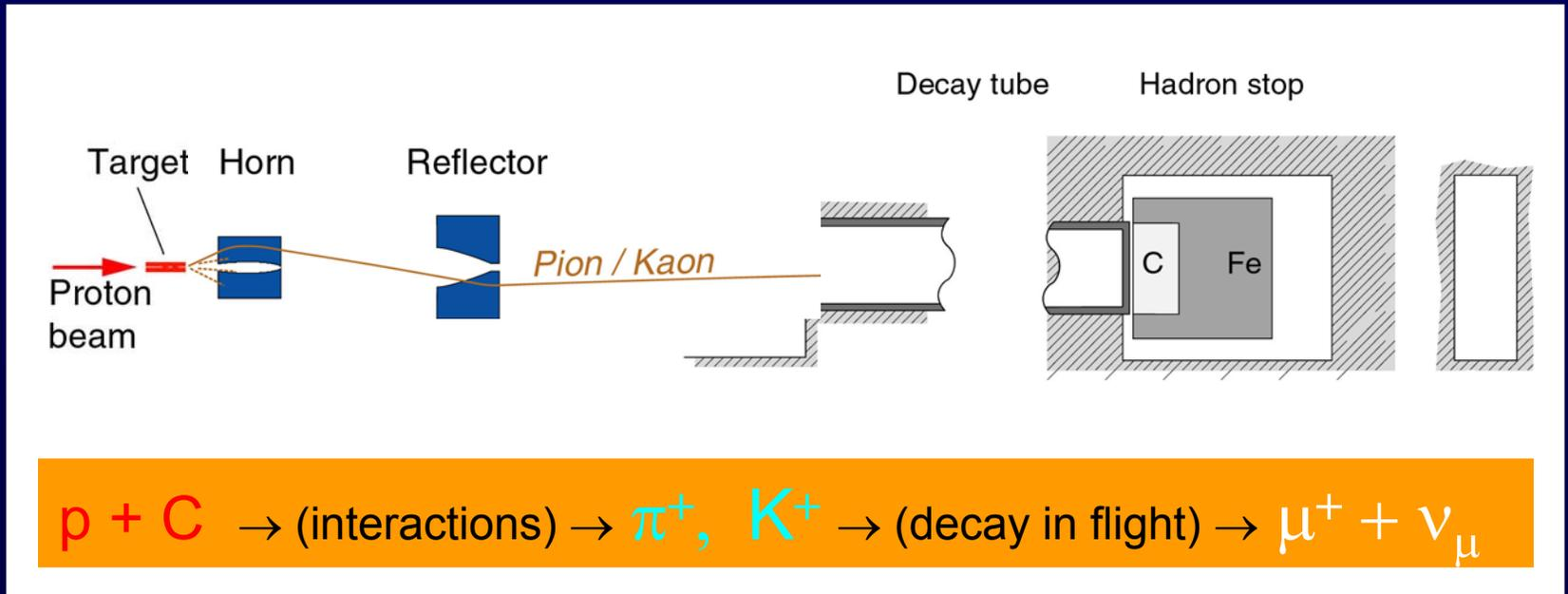
protons from SPS: 400 GeV/c, beam-size  $\sigma = 0.5\text{mm}$
