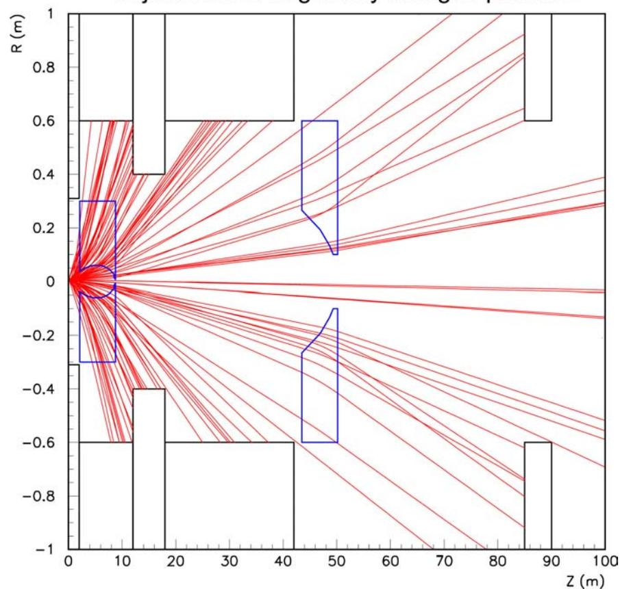
magnetic horn: pulsed -  $I = 150 \text{ kA}$ ,  $\tau = 1 \text{ ms}$
