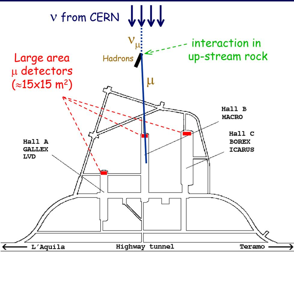
Up-stream rock --> large target mass (equivalent to tens of kt)
