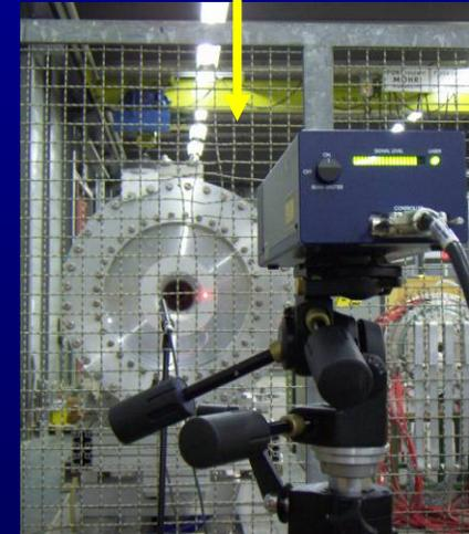
→ Natural frequency horn: 149Hz (reflector: 73Hz)
