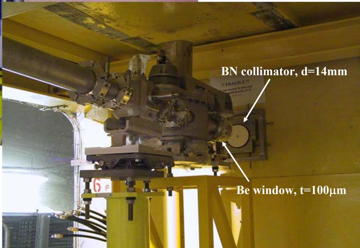
BN collimator,  $d=14\text{mm}$
