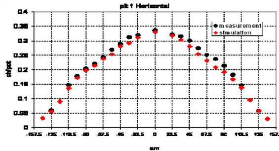
Figure 4: Measured (black circles) and simulated (red rectangles) horizontal muon profile in the first muon detector station. Each point corresponds to one ionization chamber readout.
