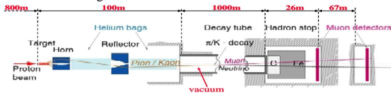
Figure 1: Main components of the CNGS facility.
