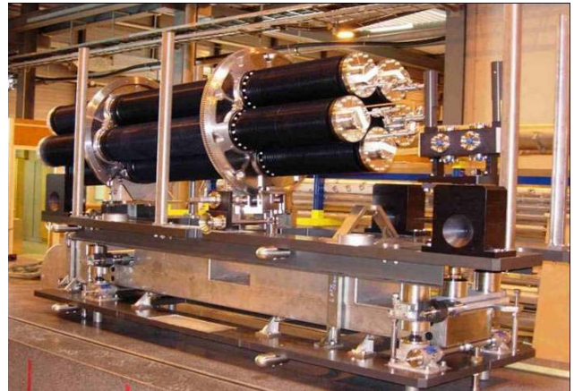
Fig. 5. CNGS target magazine consisting of five target units. Only the bottom unit is used, the other four are kept as spares.
