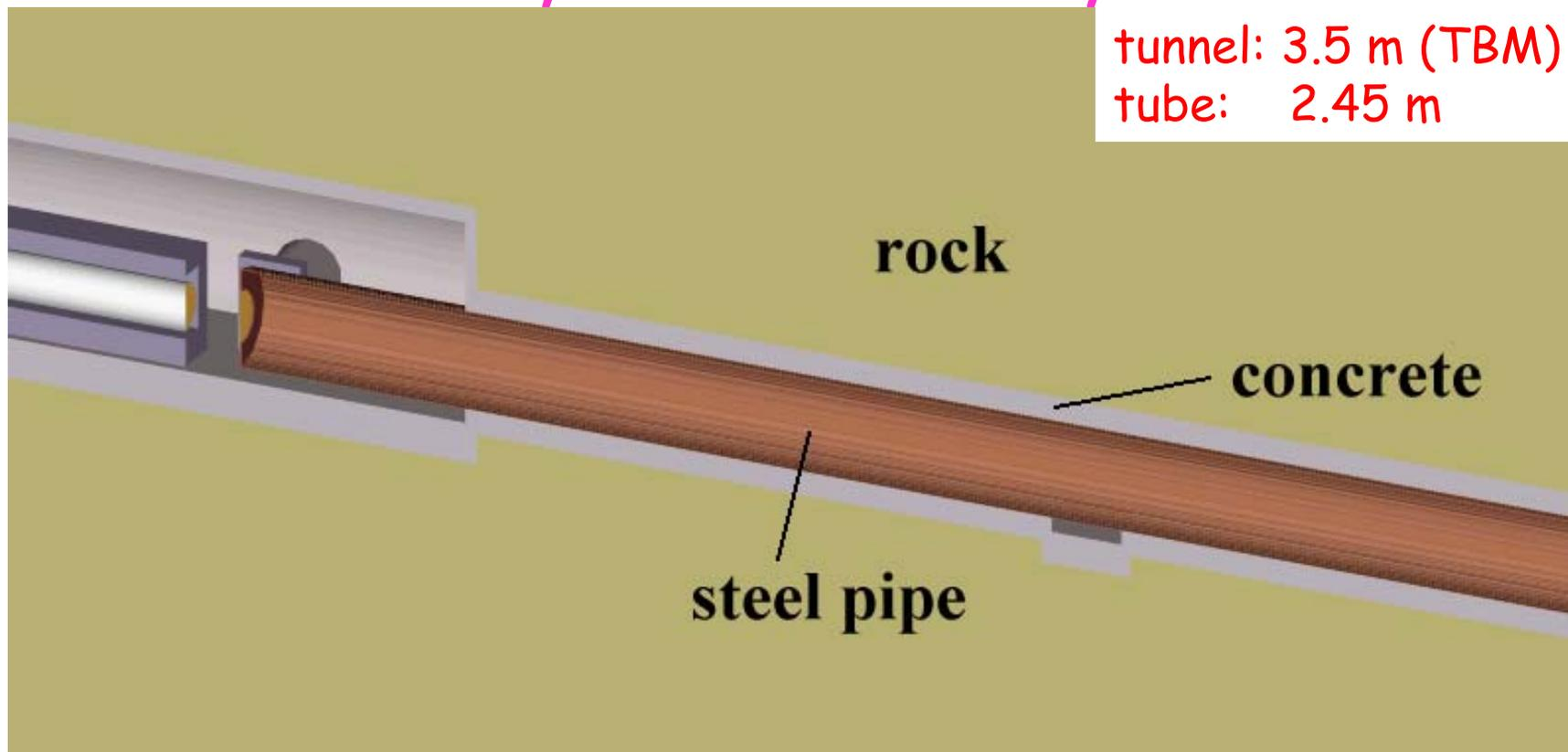
998 m long steel tube, surrounded by 50 cm of concrete
