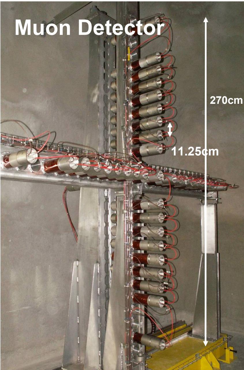
Muon detectors very sensitive to any beam change –give online feedback for neutrino beam quality!!
