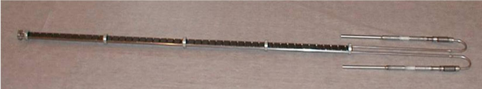
47 graphite segments, 20mm length and 6.4 x 15mm<sup>2</sup> cross-section
