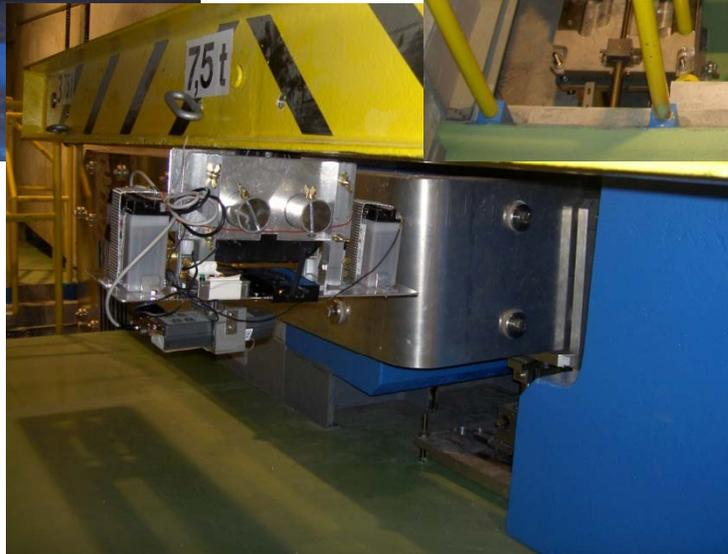
Reaches nearly any location in the target chamber. **Prevents exposure** of personnel to high radiation levels **during manual measurements.**
