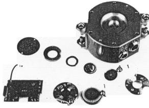
The disassembled detector mounting together with the tight box. The detector shown here, has an active area of 2 cm<sup>2</sup>.
