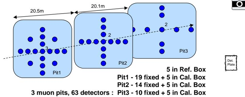
A remotely controlled girder ("lift") equipped with a calibration box was able to be positioned in front of any point of support plate. There was a space on each lift to transport at the same time a second box of the same type (reference box)
