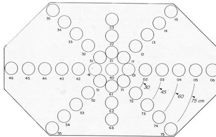
Geometry of the detector support plate. The numbers are the position indicators.
