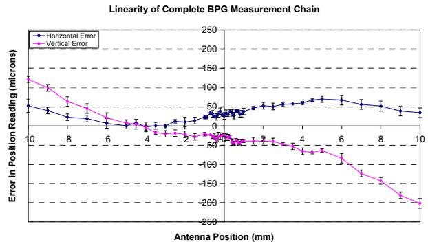
Figure 5: Laboratory Results of BPM System.
