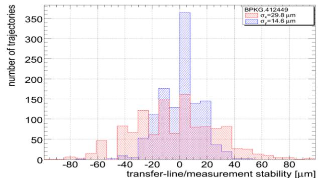
Figure 6: Stability of the target station BPM reading.
