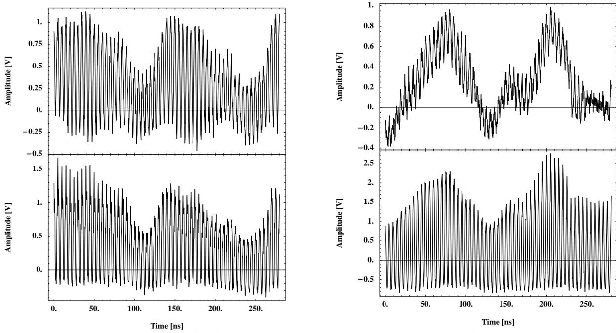
Figure 7: Bunch length along the first batch at injection (top) and 100 ms later (bottom). Conditions in the PS: beam is bunched at  $h = 16$ ; left: debunching on, modulation with seven 200 MHz cavities (nominal scheme of PS-SPS transfer); right: debunching off, modulation with one 200 MHz cavity. MD on 22.09 (left) and 30.09 (right).
