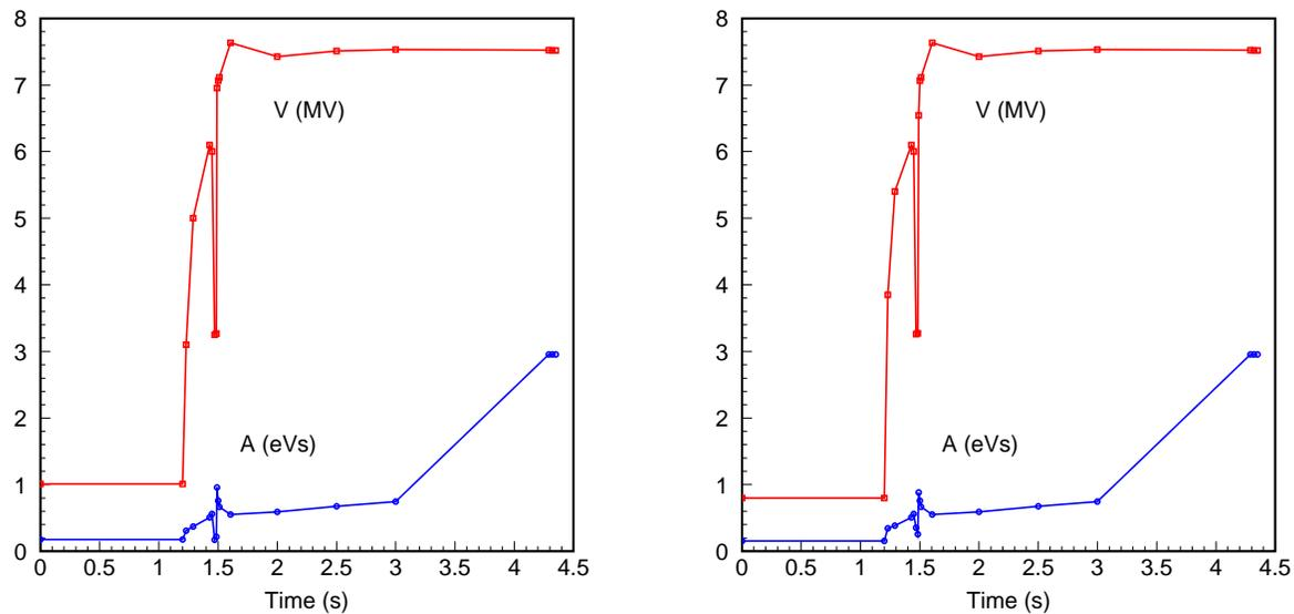
Figure 1: Voltage programme and corresponding bucket area at the beginning of the CNGS run (voltage program V-I), MD on 15.09 (left) and during normal operation, fixed target cycle (right).
