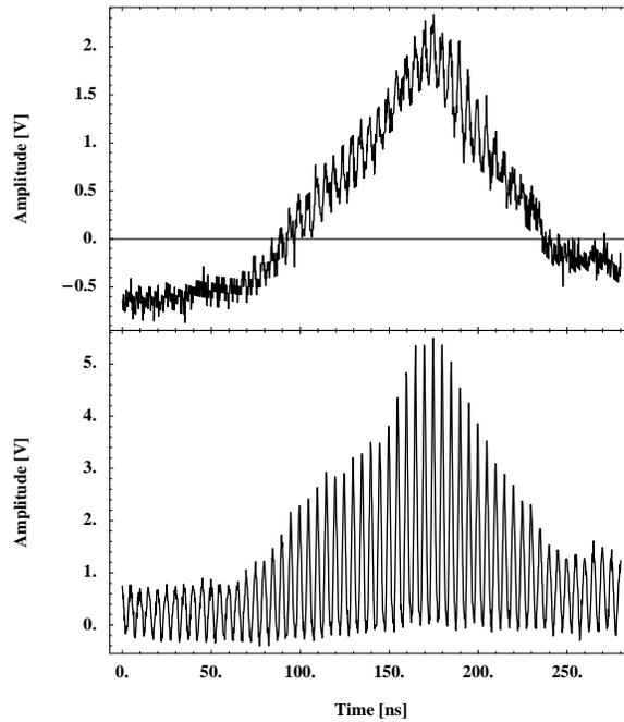
Figure 8: Bunch length along the first batch at injection (top) and 100 ms later (bottom). Conditions in the PS: beam is bunched at  $h = 8$ , debunching off, modulation with one 200 MHz cavity. MD on 1.10.
