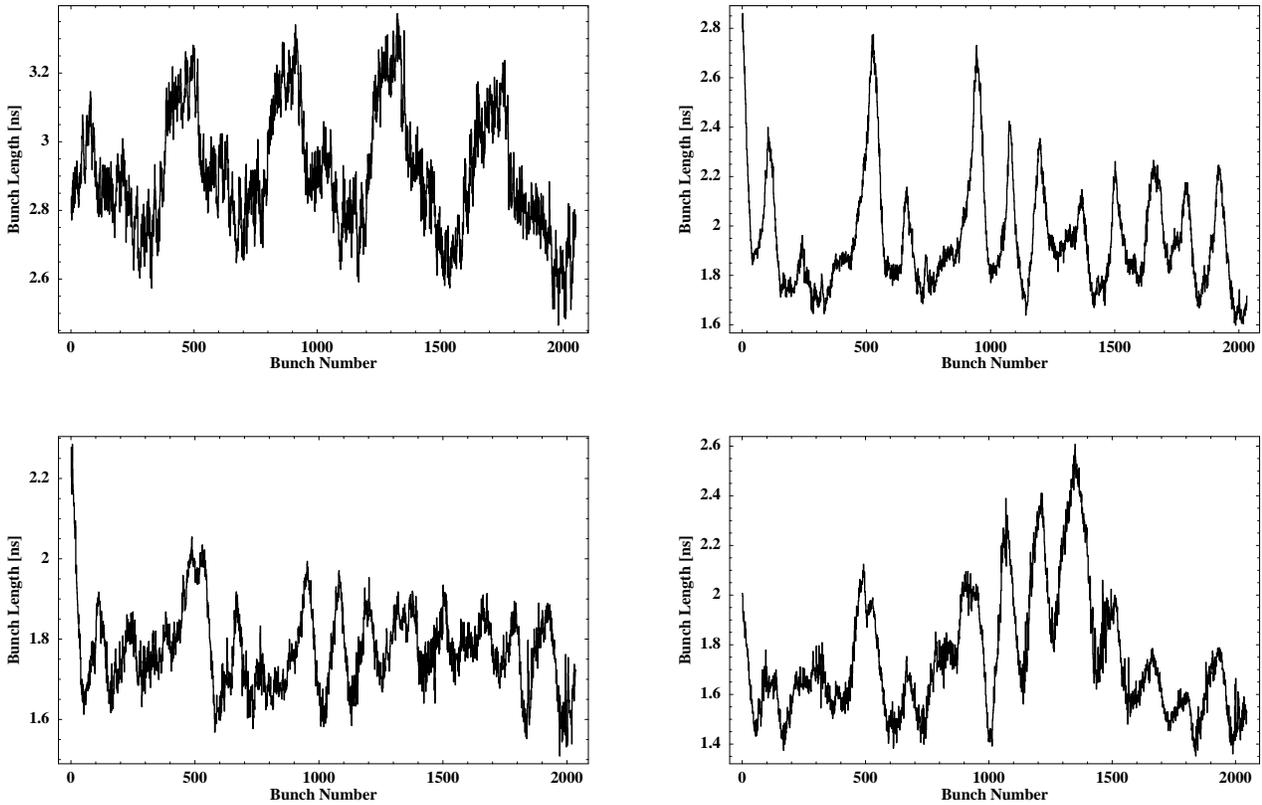
Figure 6: Bunch length as a function of bunch number in the first batch at different moments in the cycle:  $t=1.315$  s - below transition, (top, left),  $t=1.534$  s - after transition (top, right),  $t=3.286$  s (bottom, left) and  $t=4.163$  s (bottom, right). RF settings in the PS: 2.5 kV at  $h = 16$ , debunching on, full modulation at 200 MHz. MD on 30.09.
