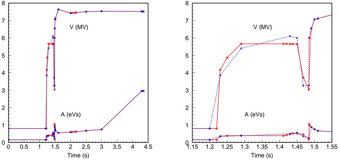
Figure 3: Voltage programme and corresponding bucket area before (V-1, dashed line) and after (V-4, solid line) trims during MD on 21.09. Whole cycle (left figure) and zoomed in around transition energy (right).
