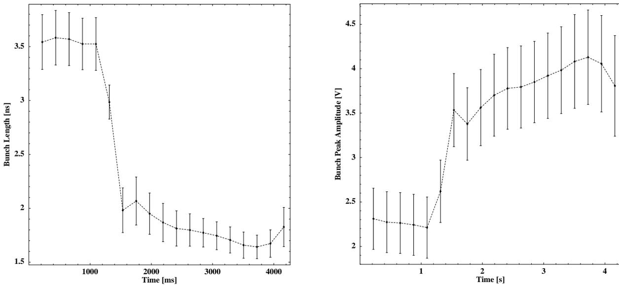
Figure 10: Bunch length (left) and peak amplitude (right) evolutions during the cycle (averaged for  $\sim 2000$  bunches of the first batch). Nominal conditions in the PS (debunching on, full modulation at 200 MHz). Increased phase loop gain in the SPS after transition (reduced losses). Beam intensity at 400 GeV:  $5.1 \times 10^{13}$ . MD on 1.10.
