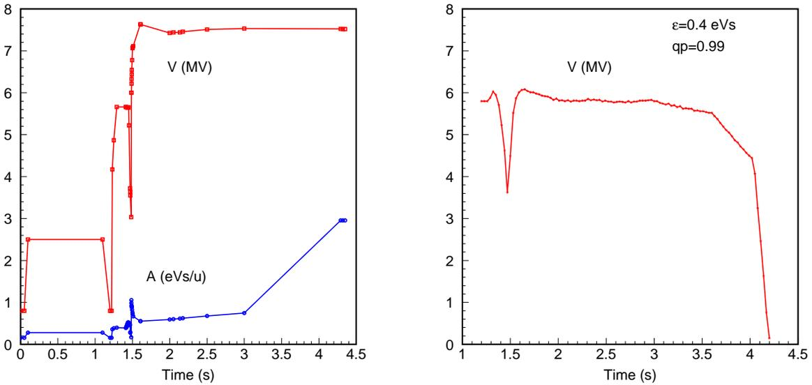
Figure 4: Left: voltage programme (V-5) and corresponding bucket area used as nominal from MD on 22.09. Right: calculated voltage programme for constant bucket area of 0.4 eVs used after transition crossing during MD on 29.09. No additional losses were observed from transition till 4 s in the cycle.
