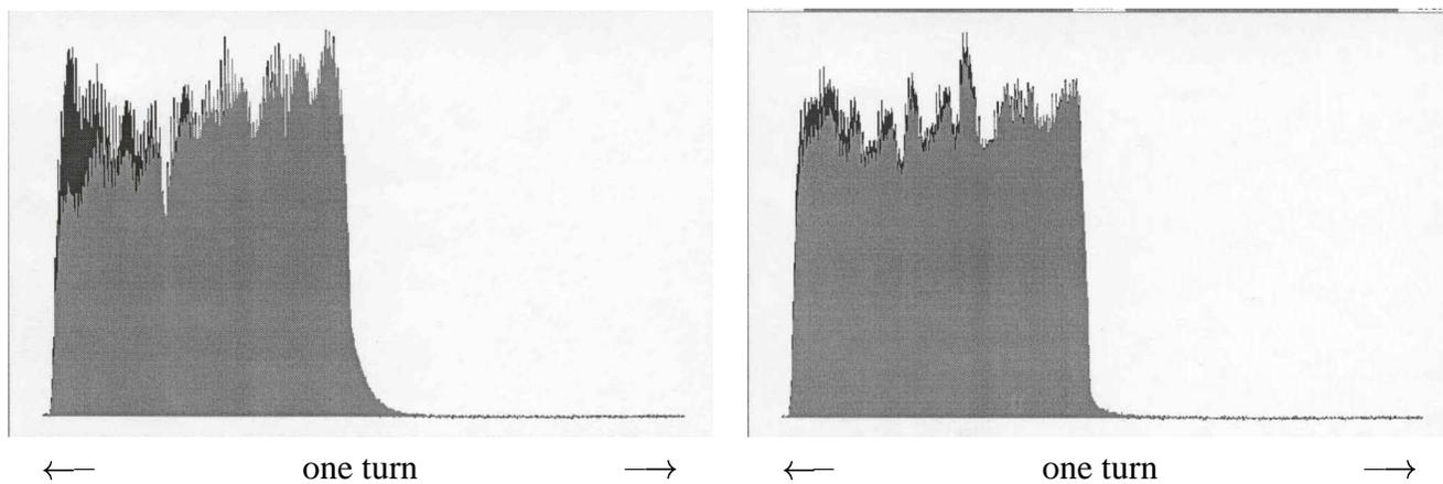
Figure 2: Fast BCT signal of the first batch at injection (black) and at the beginning of the ramp (gray) for the capture voltage of 800 kV constant (left) and increased after 50 ms to 2.5 MV in 50 ms (right). Note triangular batch shape and recaptured particles in the kicker gap for the first case. MD on 15.09 (left) and 22.09 (right).
