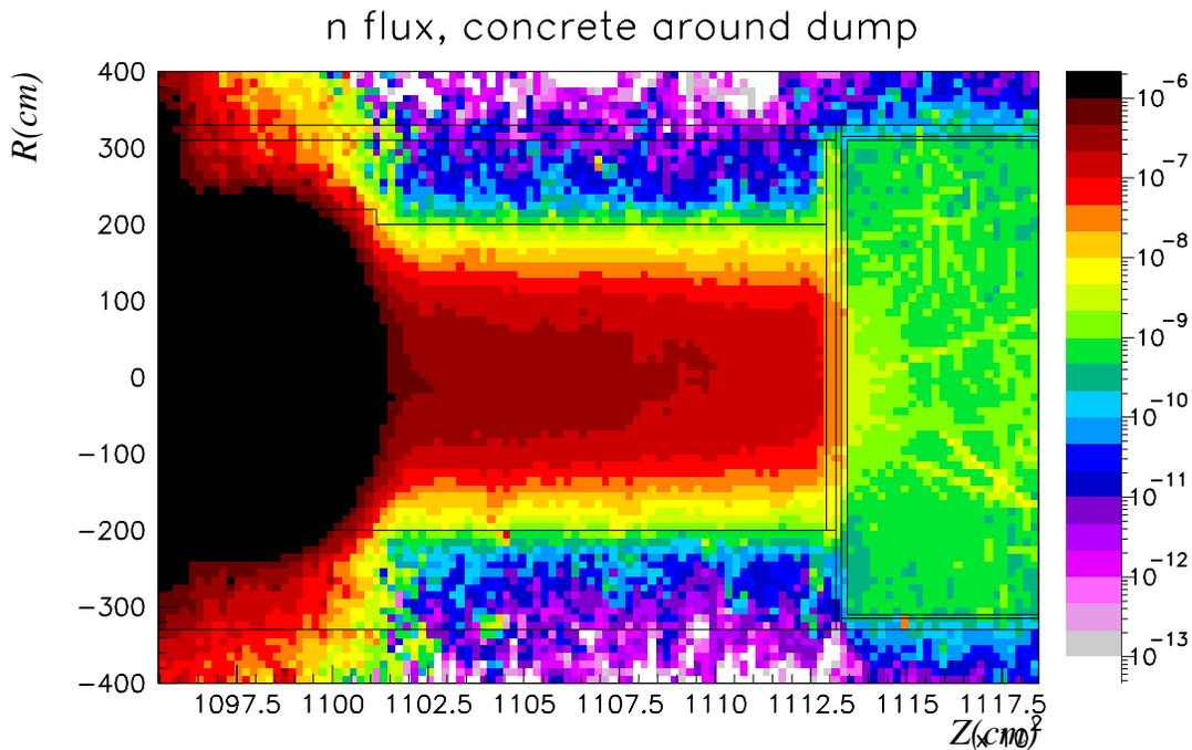
Figure 3: Neutron flux in a vertical section of the dump cavern, in the present layout (top) and in the old layout (all space filled with concrete).
