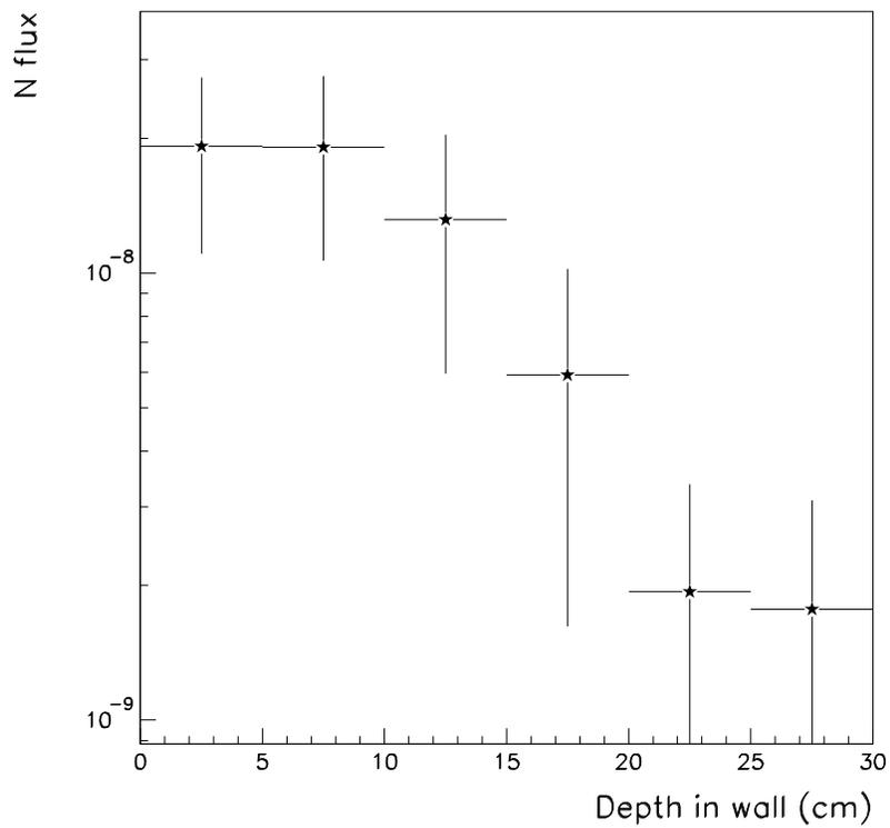
Figure 8: Longitudinal profile of neutron flux inside the concrete wall that separates dump and pit. Flux is integrated over energy and transversal dimensions.
