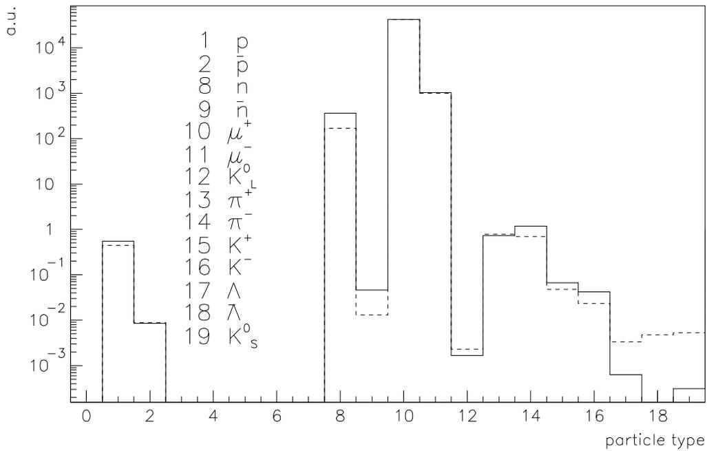
Figure 5: Particle spectrum at the first pit: standard case “air” (full line) compared to “concrete” case (dashed line).
