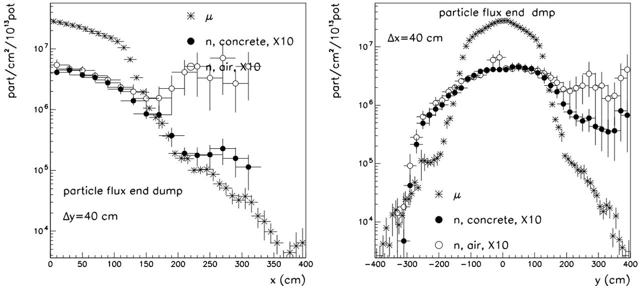
Figure 4: Muon and neutron fluxes at the end of the beam-dump cave, in the the horizontal (x, right) and vertical(y, left) plane, calculated in the standard dump configuration (air) and with the space between iron absorber and cavern wall filled with concrete (concrete). Fluxes are averaged over  $\pm 20 \text{ cm}$  in  $y$  (resp.  $x$ ). Neutron fluxes are multiplied by 10.
