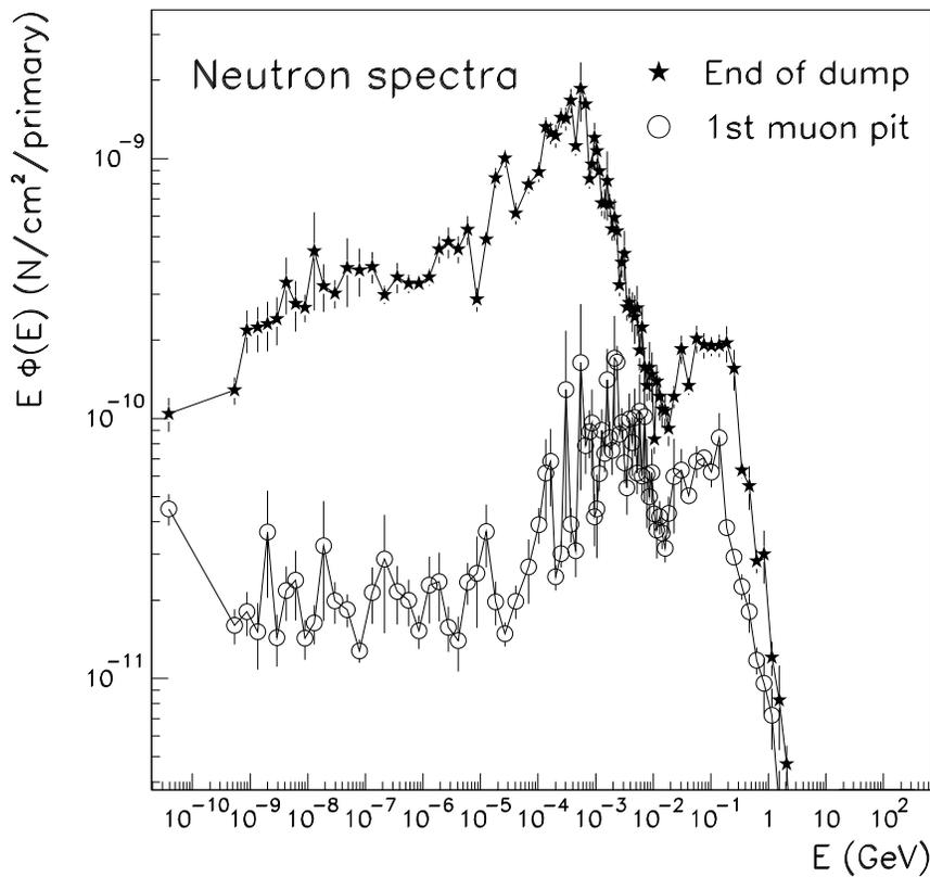
Figure 7: Lethargy neutron spectra at the end of dump and in the 1st muon pit.
