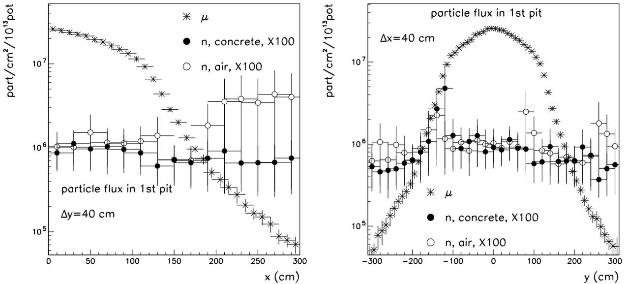
Figure 6: Muon and neutron fluxes at the entrance of the 1st muon pit. As in fig. 4, but neutron fluxes are multiplied by 100.
