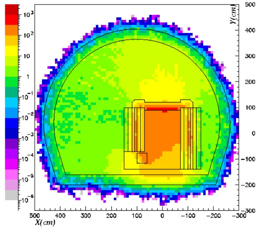
Figure 11 Dose equivalent rate (mSv/h) after a cooling time of two months
