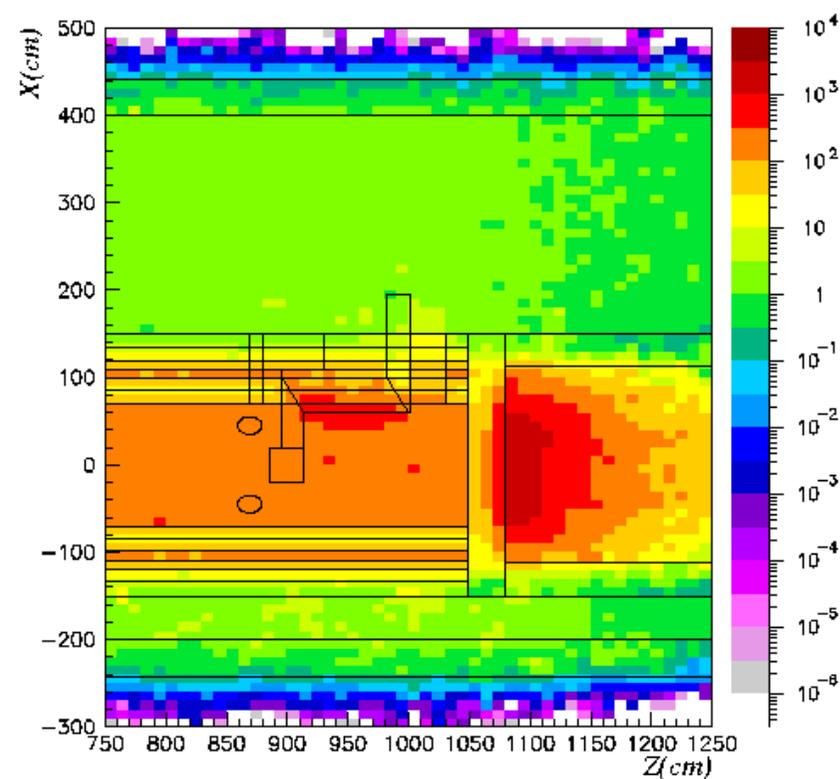
Figure 30 Total dose equivalent rates after a cooling time of 1 week
