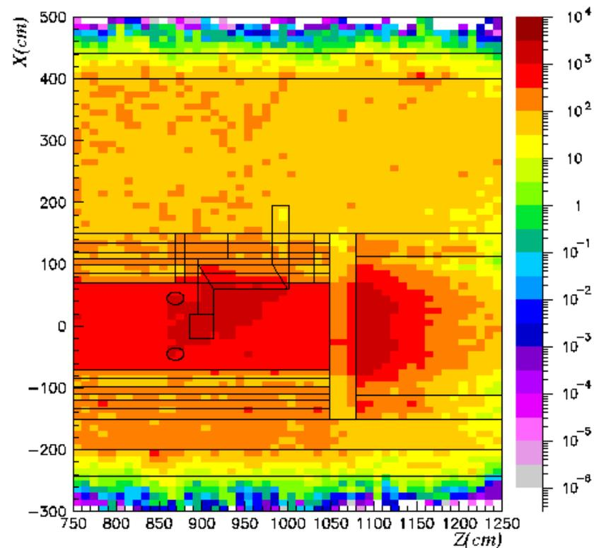
Figure 39 Total dose equivalent rates after a cooling time of 1 day
