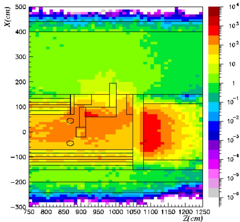
Figure 22 Total dose equivalent rates after a cooling time of 1 month
