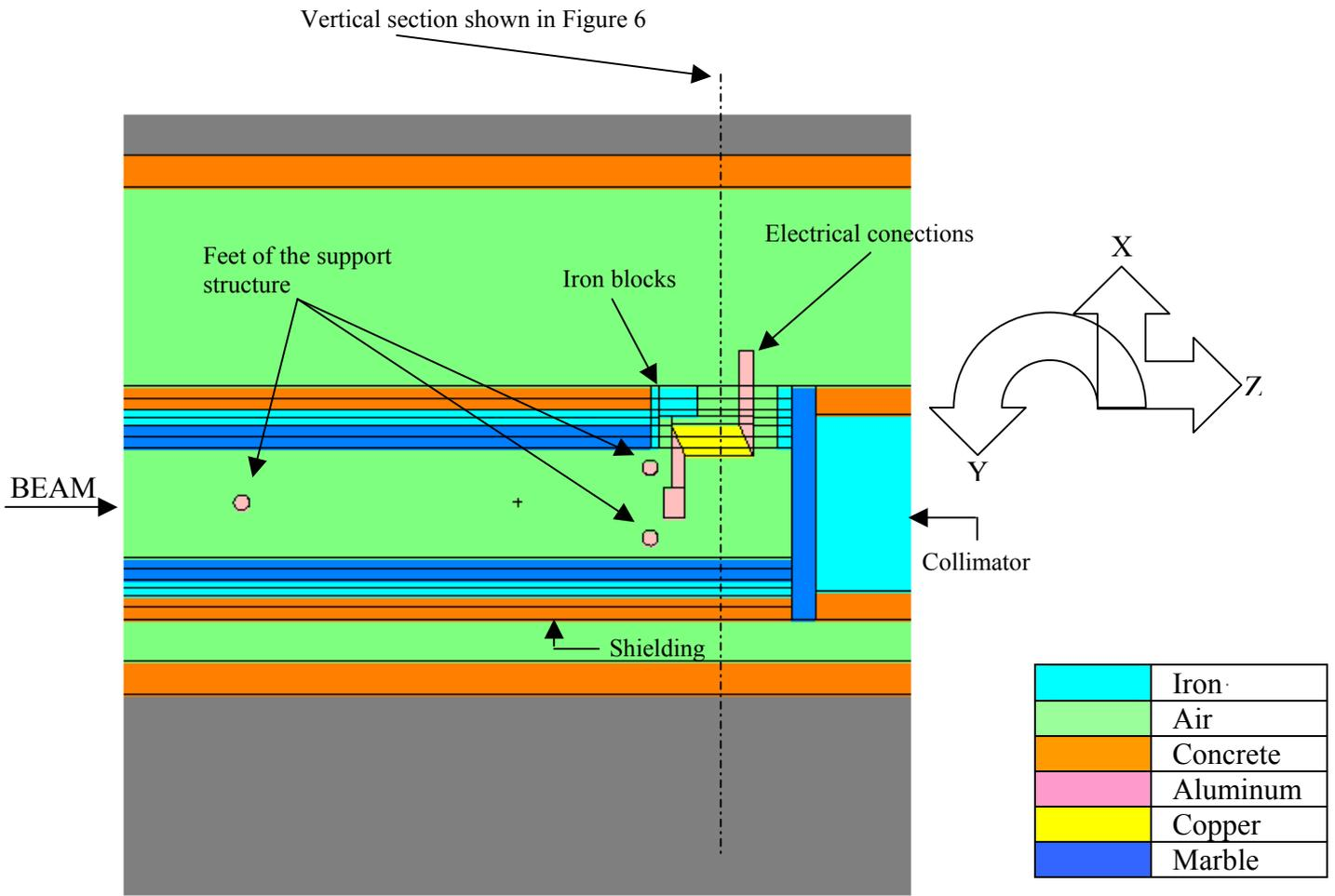
**Figure 7 Horizontal longitudinal section at the height of the FCS ( $y = -90$  cm)**
