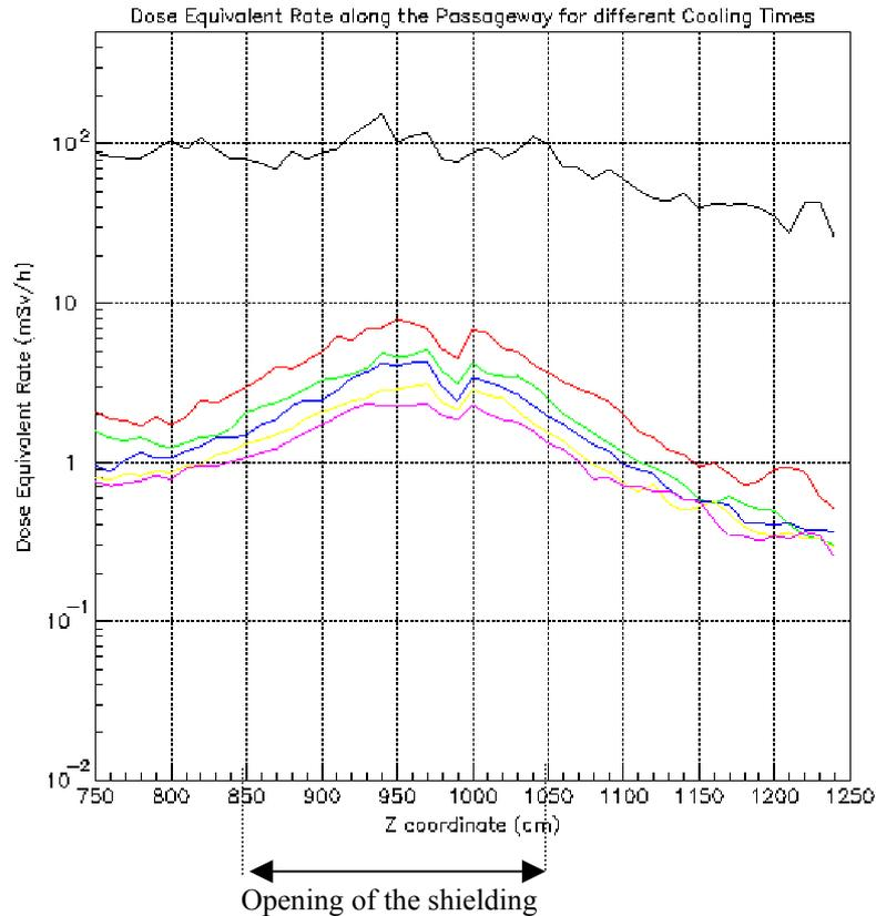
**Figure 27** Average values in a bin centered at  $y=-90$  cm (20cm long),  $x=200$  cm (40 cm long), in black after a cooling time of 1 day and the other colors after cooling times of 1 week, 1 month, 2 months, 4 months and 6 months
