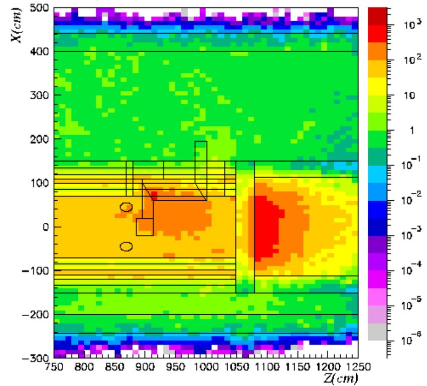
Figure 32 Total dose equivalent rates after a cooling time of 2 months
