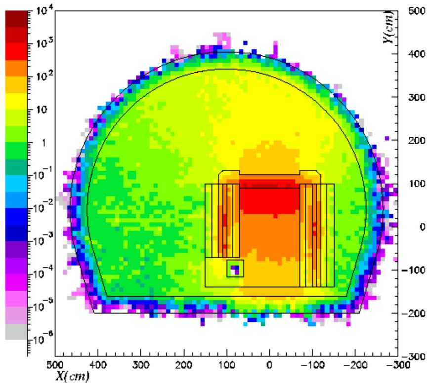
Figure 14 Shielding contribution (mSv/h) after a cooling time of one week
