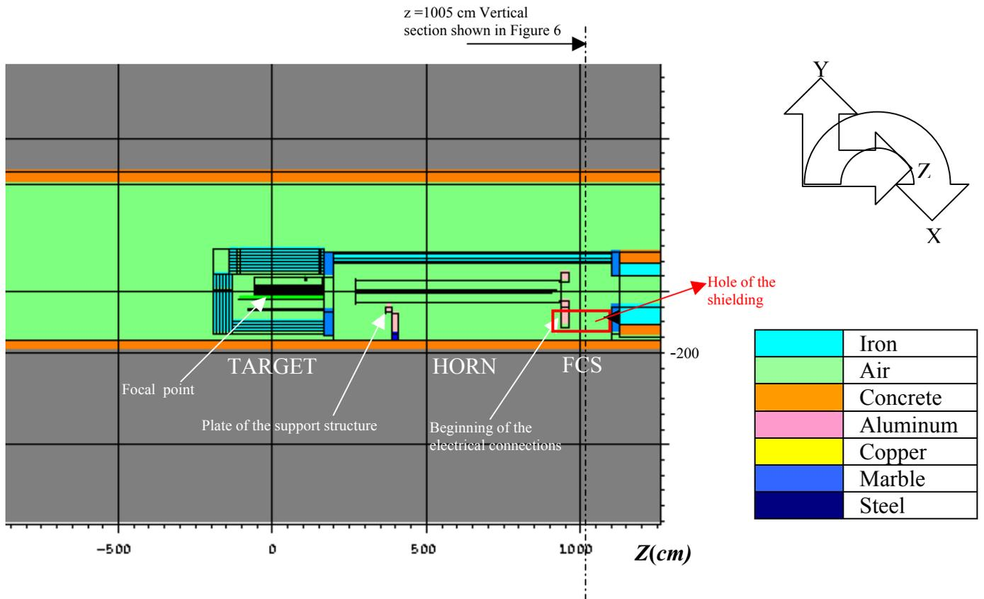
**Figure 5: Vertical longitudinal section through the FLUKA geometry of target and horn**
