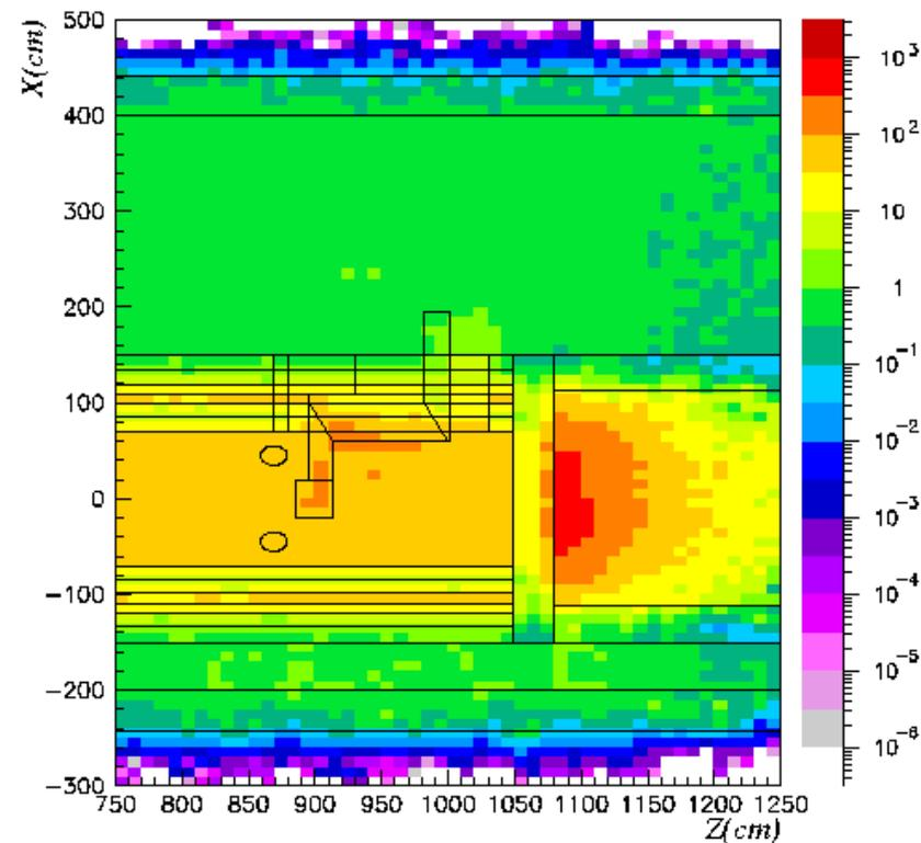
Figure 34 Total dose equivalent rates after a cooling time of 6 months
