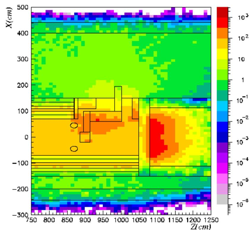
Figure 23 Total dose equivalent rates after a cooling time of 2 months
