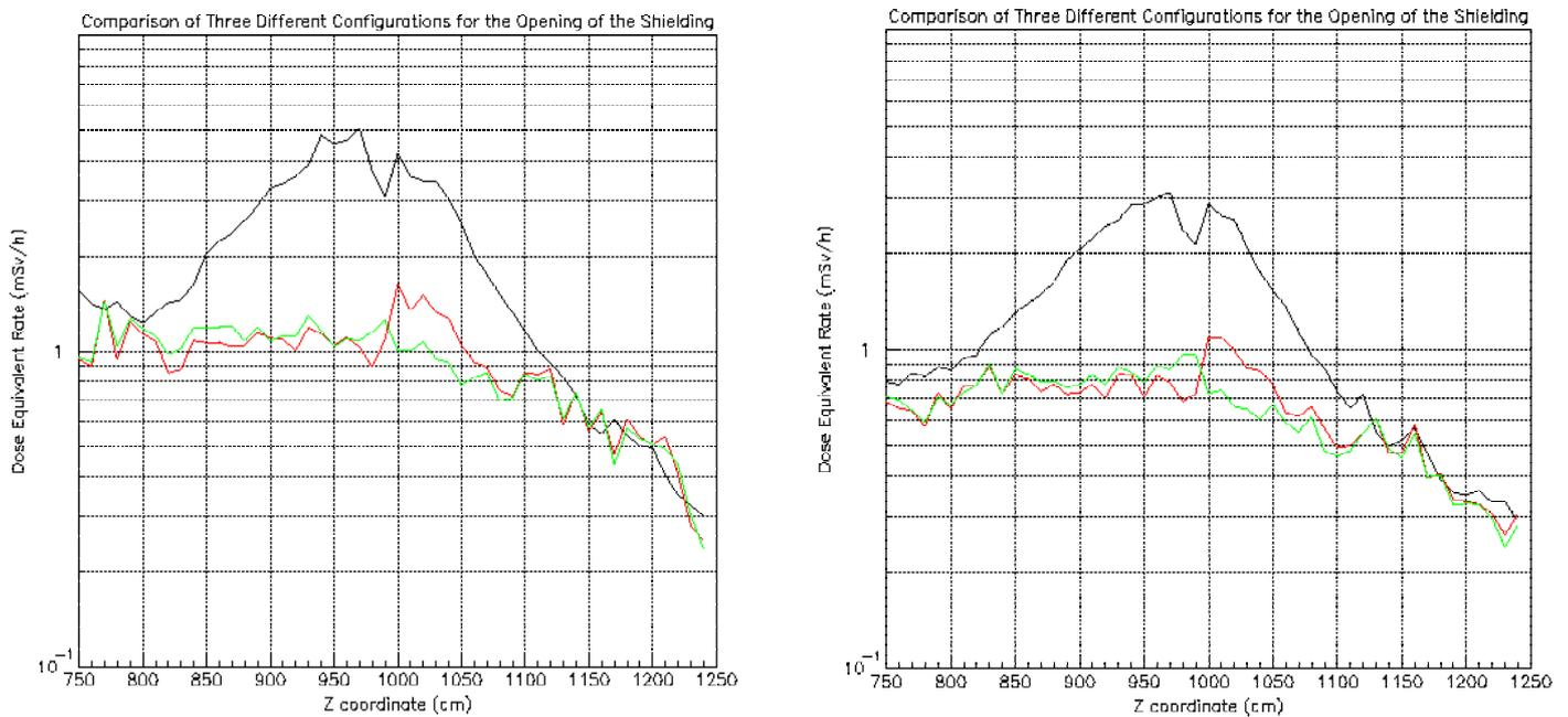
Figure 38 Average values in a bin centered at  $y=-90$  cm (20cm long),  $x=200$  cm (40 cm long) along the passageway, in black the layout of Figure 7, in red the layout of Figure 28 and in green the layout of Figure 36 after a cooling time of 1 month (left) and after a cooling time of 4months (right).
