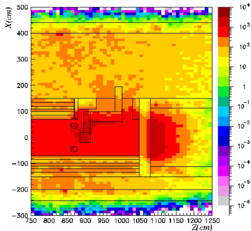
Figure 20 Dose equivalent rate after a cooling time of 1day
