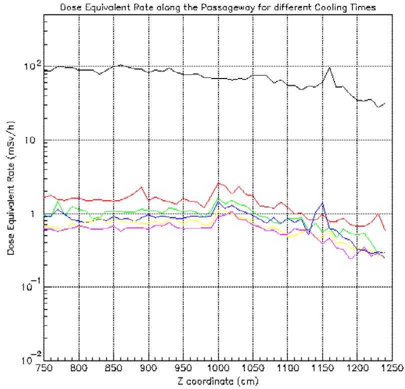
**Figure 35 Average values in a bin centered at y=-90 cm (20cm long), x=200 cm (40 cm long), in black after a cooling time of 1 day and the other colors after cooling times of 1 week, 1 month, 2 months, 4 months and 6 months**
