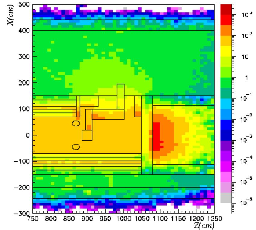
Figure 25 Total dose equivalent rates after a cooling time of 6 months
