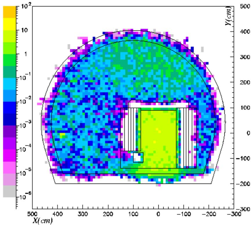
Figure 16 Collimator contribution (mSv/h) after a cooling time of one week
