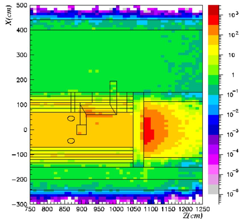
Figure 44 Total dose equivalent rates after a cooling time of 6 months
