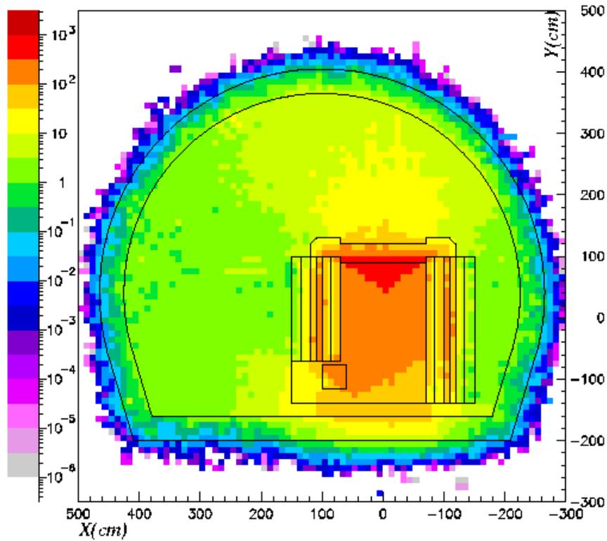
Figure 10 Dose equivalent rate (mSv/h) after a cooling time of one month
