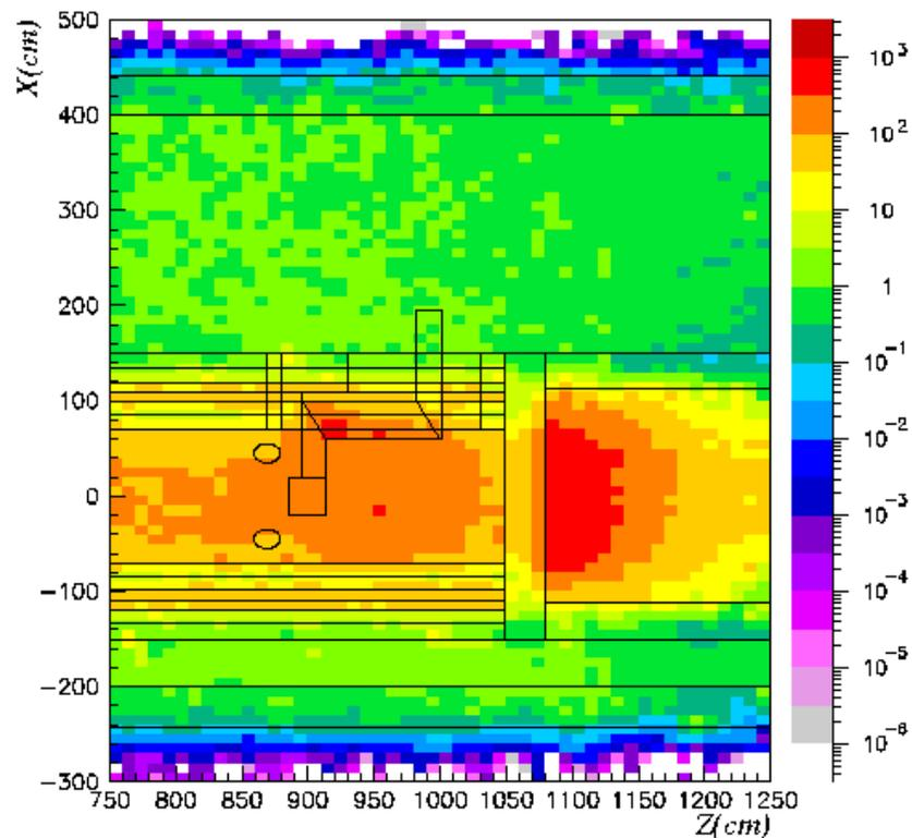
Figure 41 Total dose equivalent rates after a cooling time of 1 month
