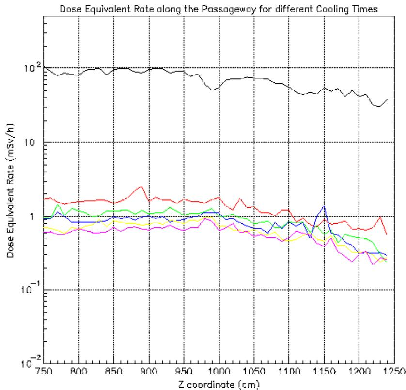
Figure 45 Average values in a bin centered at  $y=-90$  cm (20cm long),  $x=200$  cm (40 cm long), in black after a cooling time of 1 day and the other colors after cooling times of 1 week, 1 month, 2 months, 4 months and 6 months
