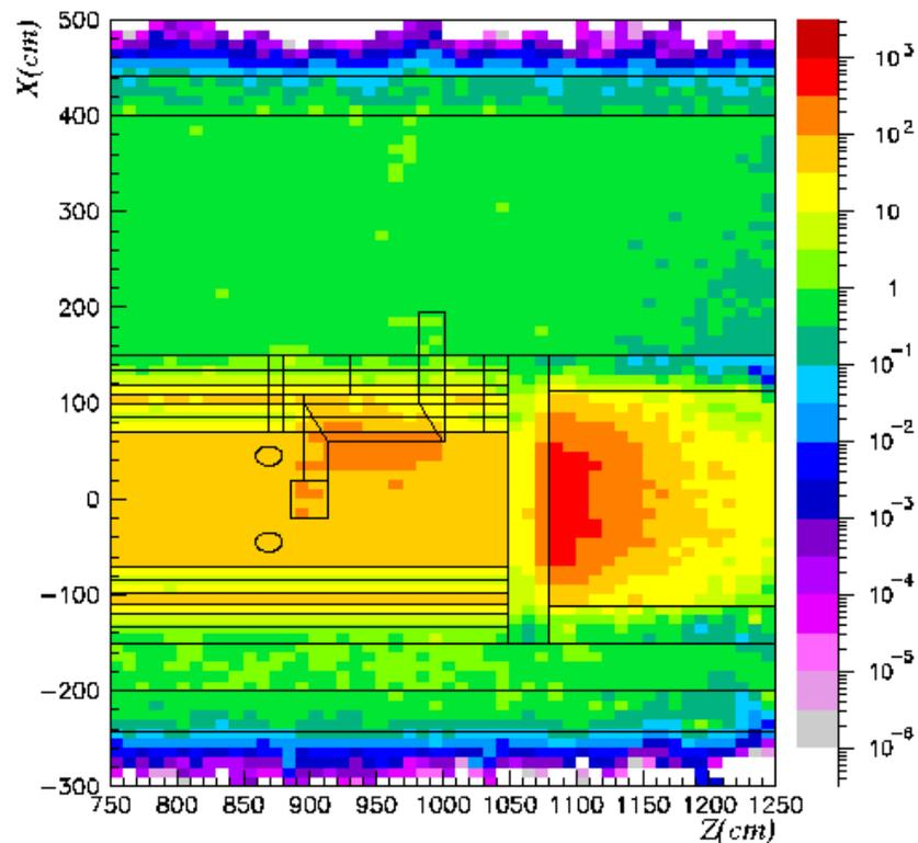
Figure 43 Total dose equivalent rates after a cooling time of 4month
