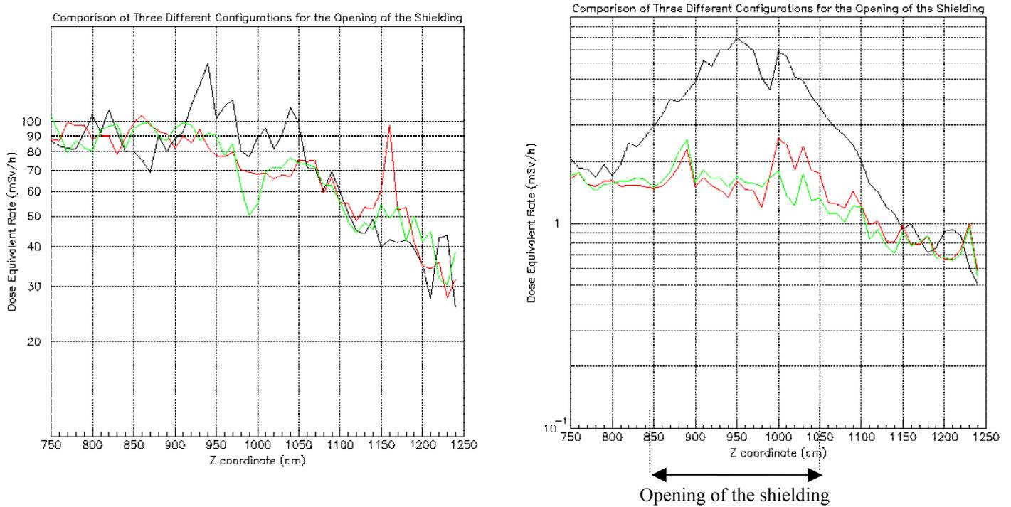
Figure 37 Average values in a bin centered at  $y=-90$  cm (20cm long),  $x=200$  cm (40 cm long) along the passageway, in black the layout of Figure 7, in red the layout of Figure 28 and in green the layout of Figure 36 after a cooling time of 1 day (left) and after a cooling time of 1 week (right).
