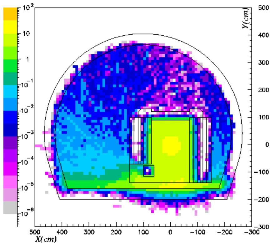
Figure 18 Collimator contribution (mSv/h) after a cooling time of one week
