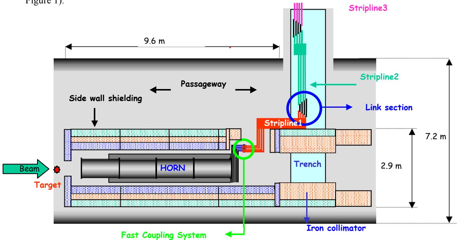
Figure 1: Schematic view (top view) of the horn region
