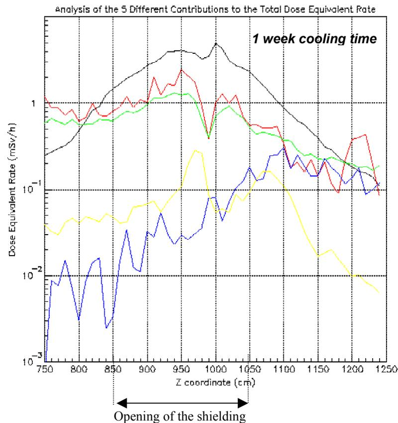
Figure 19 Comparison among different contributions along the passageway, average values in a bin centered at  $y=-90$  cm (20cm long) and  $x=200$  cm (40 cm long). In black contribution of the opening of the shielding, in red contribution of the shielding, in green contribution of the concrete wall/floor, in yellow contribution of the horn tube and in blue the contribution of the collimator.
