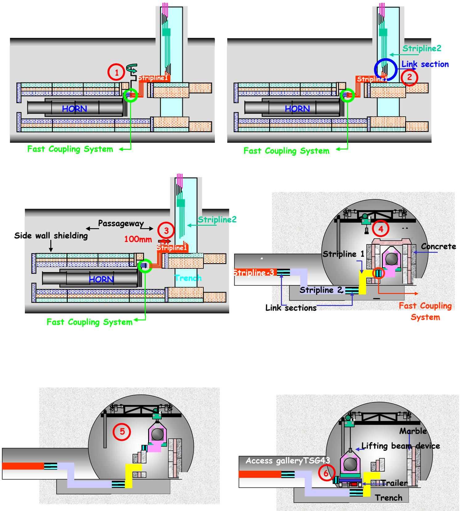
Figure 3 Sequence of steps necessary to replace the horn
