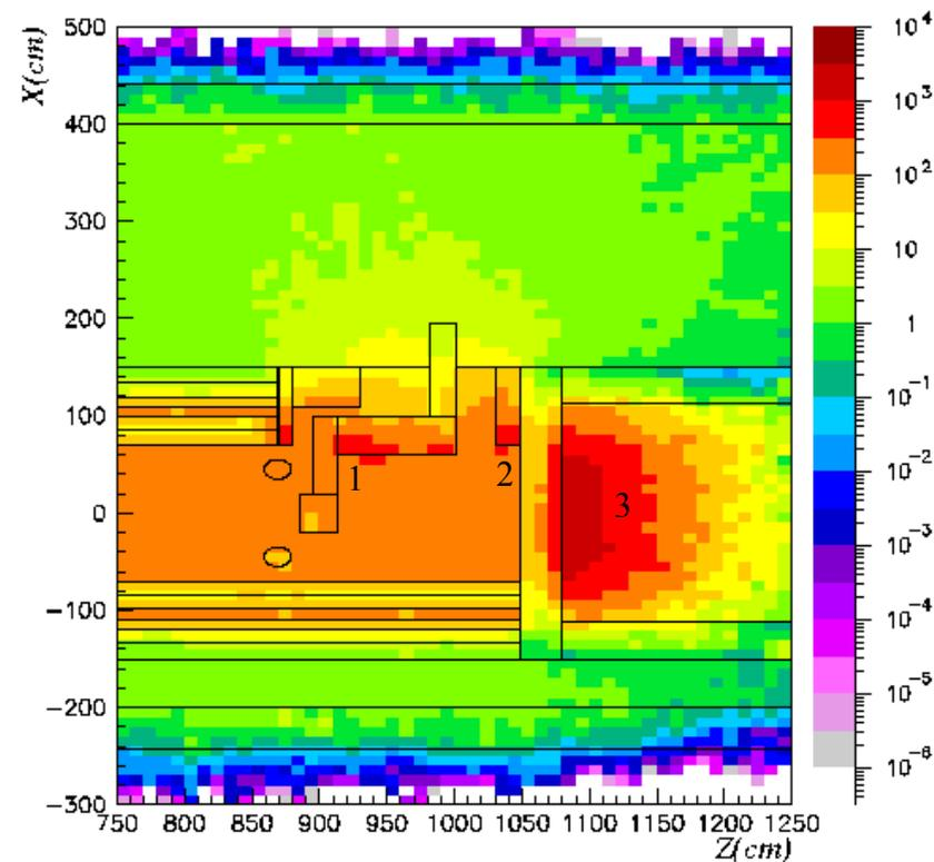
Figure 21 Dose equivalent rate after a cooling time of 1 week
