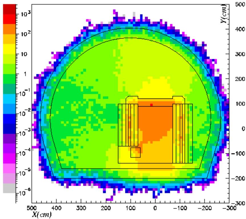
Figure 12 Dose equivalent rate (mSv/h) after a cooling time of four months
