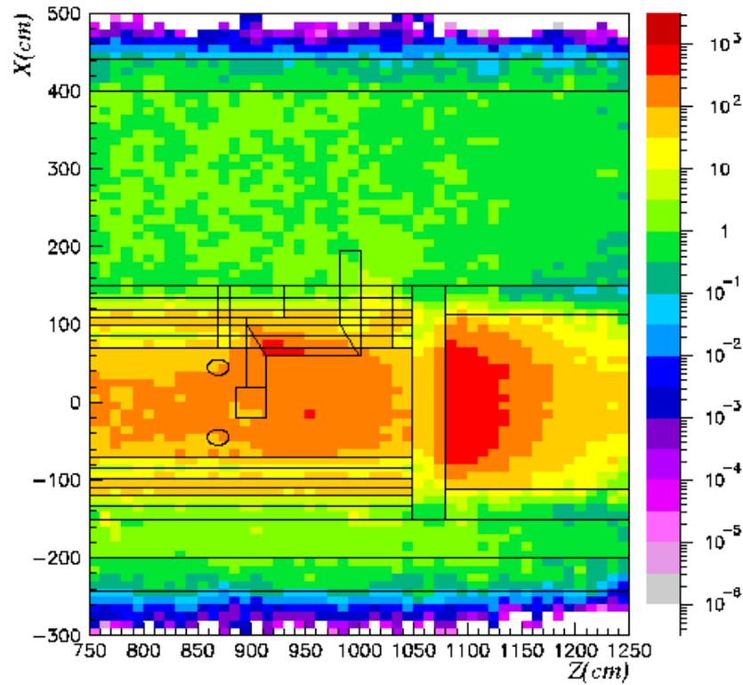
Figure 31 Total dose equivalent rates after a cooling time of 1 month
