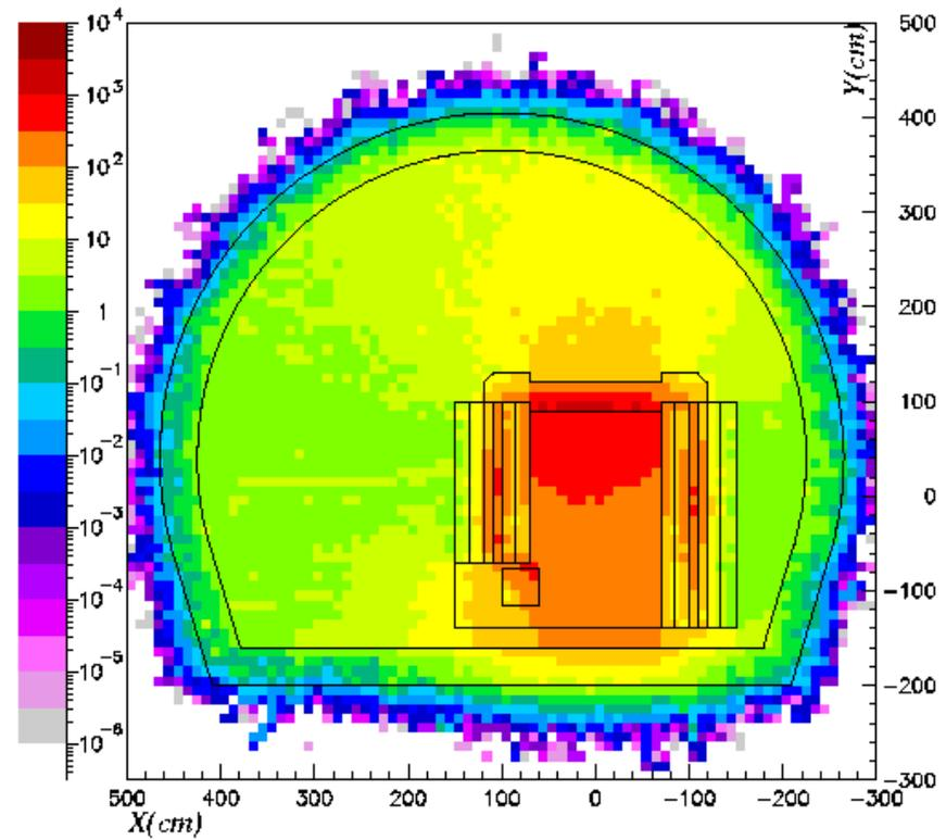
Figure 9 Dose equivalent rate (mSv/h) after a cooling time of one week
