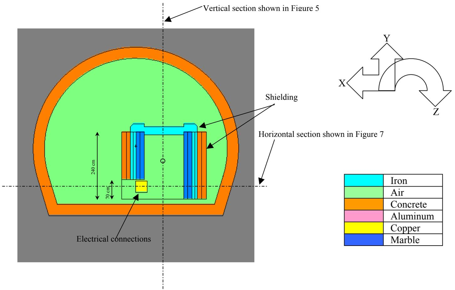
**Figure 6 Vertical transverse section at the location of the FCS (z=1005cm)**
