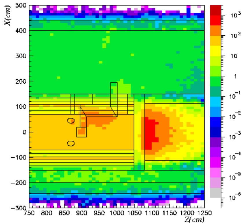
Figure 33 Total dose equivalent rates after a cooling time of 4month
