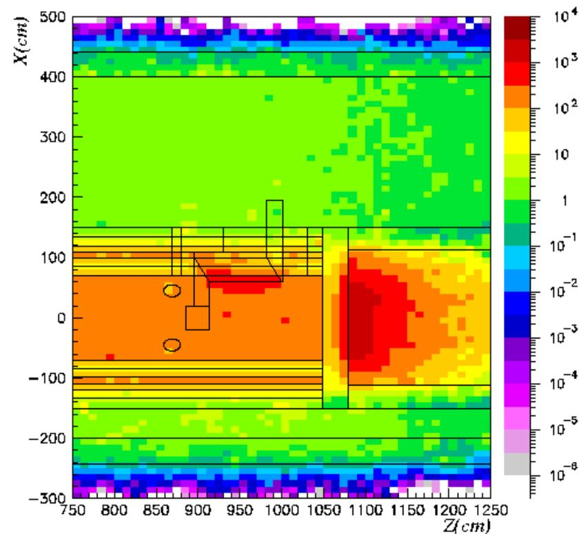
Figure 40 Total dose equivalent rates after a cooling time of 1 week
