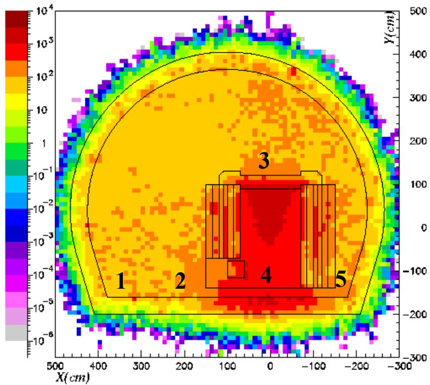
Figure 8 Dose equivalent rate (mSv/h) after a cooling time of one day
