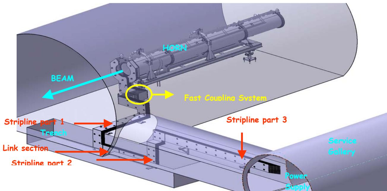
Figure 2 Artistic view of the fast coupling system region, this view does not show the shielding of the horn (Courtesy M. Briere/LAL)
