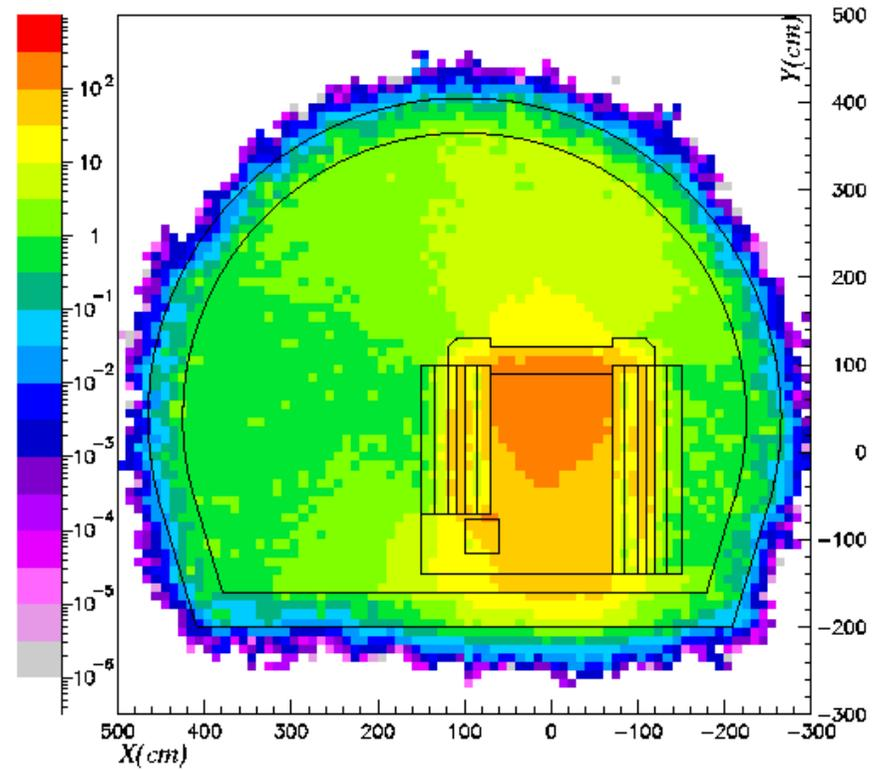
Figure 13 Dose equivalent rate (mSv/h) after a cooling time of six months
