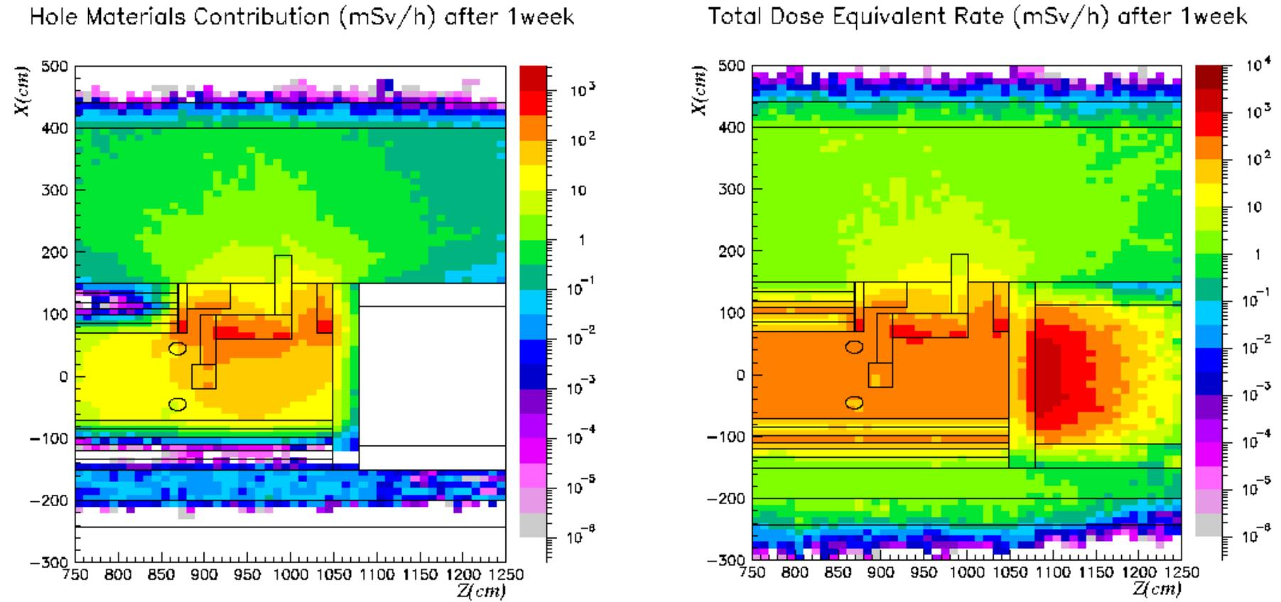
Figure 26 Comparison between the dose rate contribution of the materials inside the hole (left side) and the sum of all contributions (right side)
