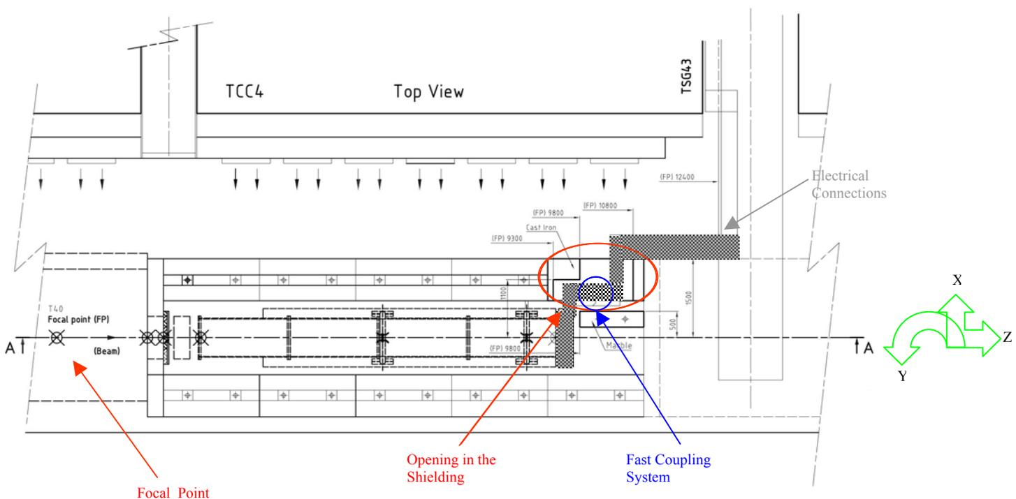
Figure 4: Present layout of the horn area
