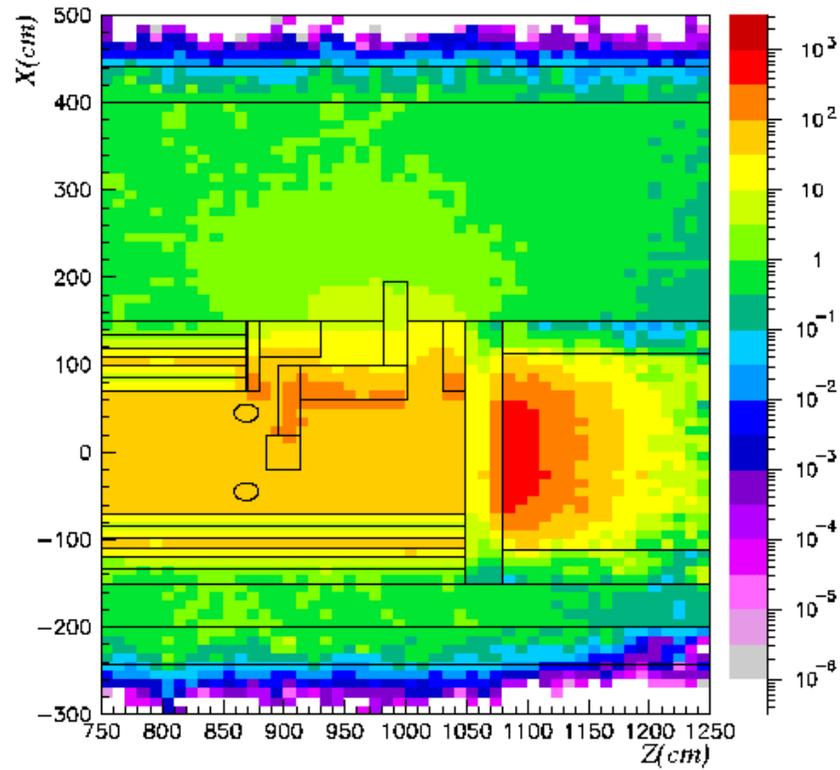
Figure 24 Total dose equivalent rates after a cooling time of 4month
