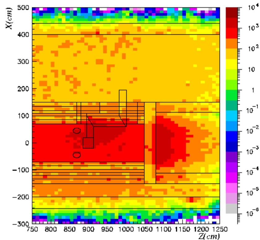
Figure 29 Total dose equivalent rates after a cooling time of 1 day
