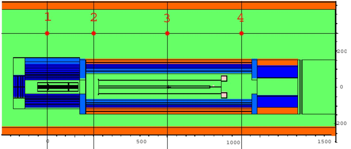
Figure 14 Horizontal longitudinal section at y=0 cm showing the locations for which dose equivalent rates are given in table 3
