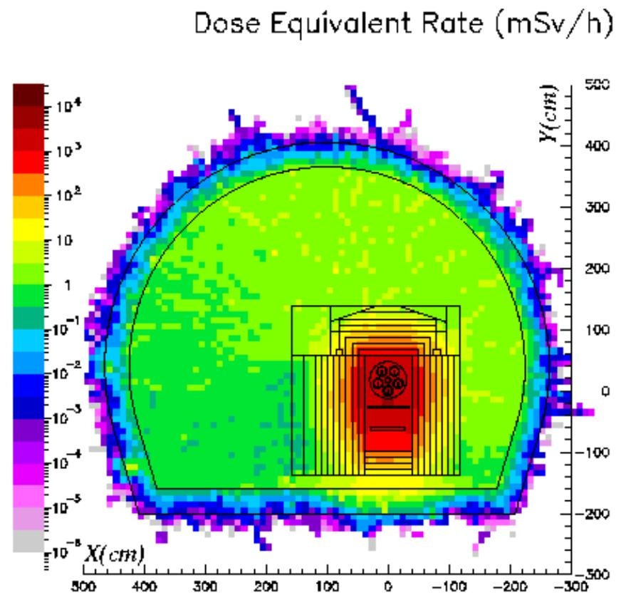
Figure 20 Total dose equivalent rate (mSv/h) after a cooling time of one week
