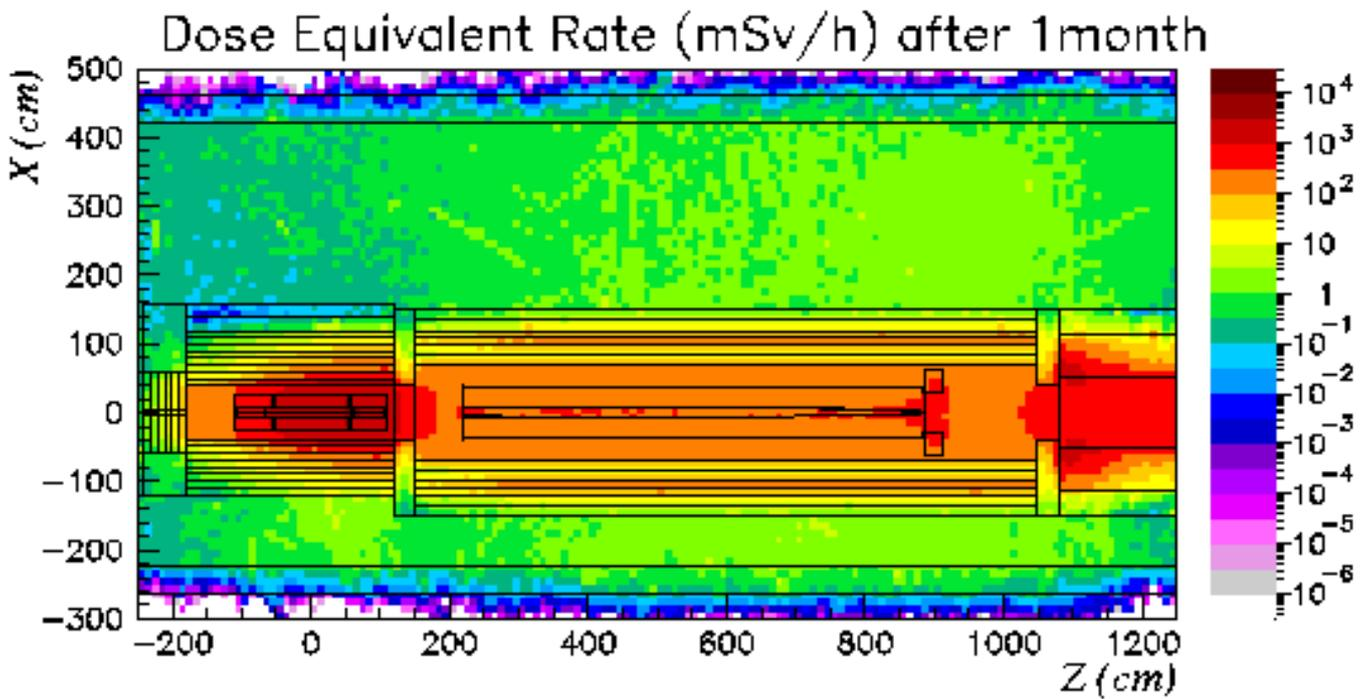
Figure 6 Total dose equivalent rate for cooling times of 1 week and 1 month for a longitudinal horizontal section at the level of the beam axis
