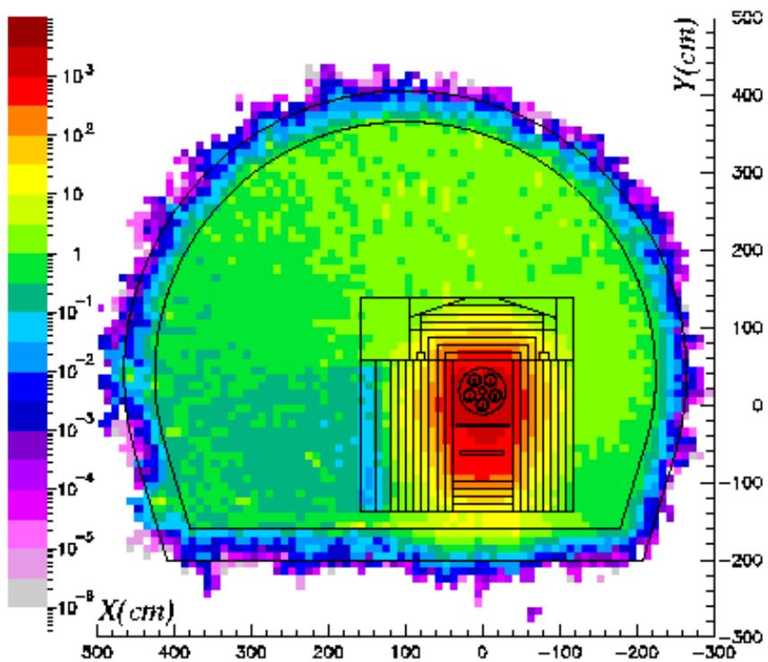
Figure 21 Total dose equivalent rate (mSv/h) after a cooling time of one month
