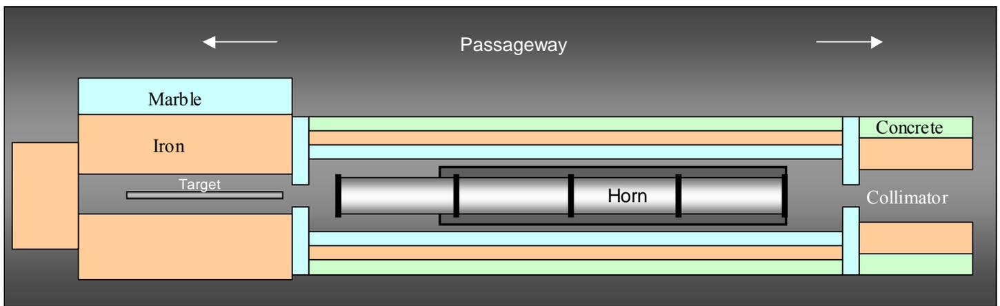
Figure 1 Schematic view of the target and horn area
