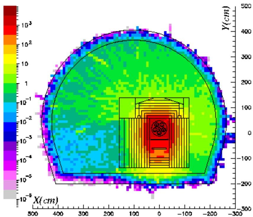
Figure 27 Target shielding contribution after a cooling time of one week
