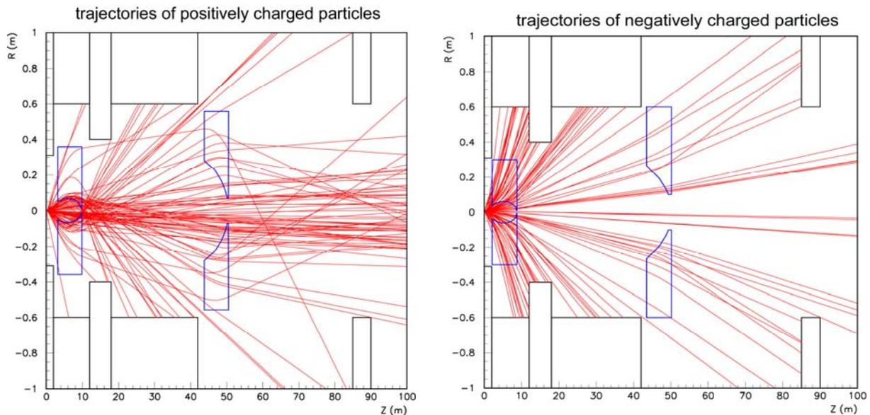
Figure 4 Trajectories of primary and secondary particles generated in the nuclear cascade
