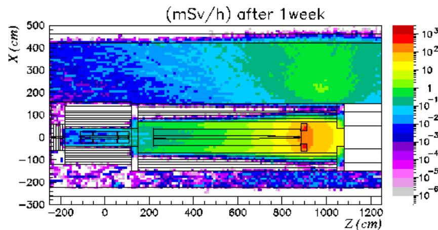
Figure 17 Dose equivalent rate from the stripline and elements of the shielding opening contribution
