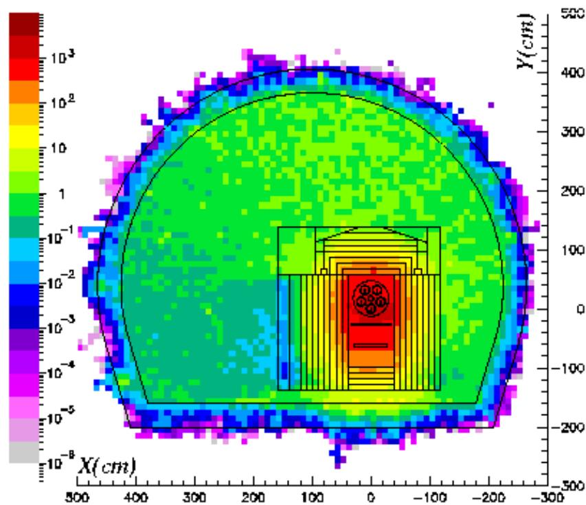
Figure 22 Total dose equivalent rate (mSv/h) after a cooling time of two months
