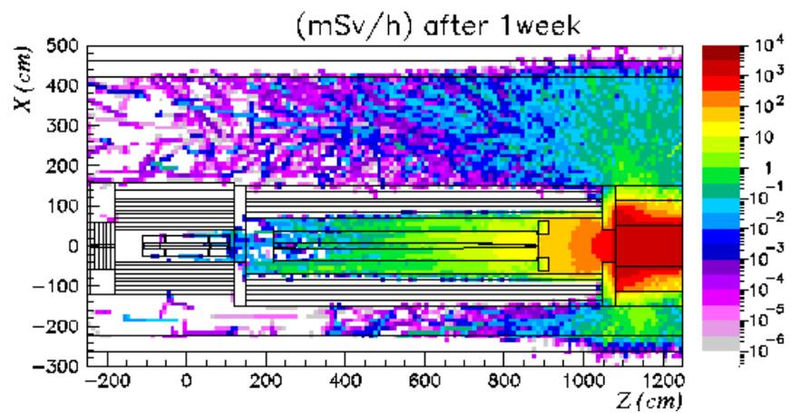
Figure 18 Dose equivalent rate of the collimator contribution
