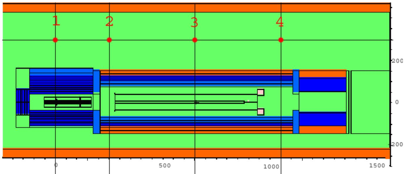
Figure 9 Horizontal longitudinal section at  $y=0$  cm showing the locations for which dose equivalent rates are given in table 2
