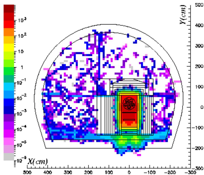
Figure 28 Target tube and adjacent materials contribution (mSv/h) after a cooling time of one week
