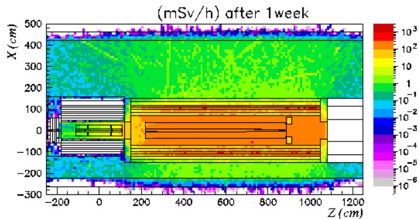
Figure 15 Dose equivalent rate from the horn shielding contribution
