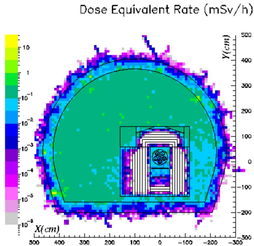
Figure 26 Wall/Floor contribution (mSv/h) after a cooling time of one week
