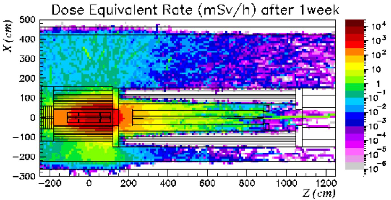
Figure 12 Contribution of the target shielding
