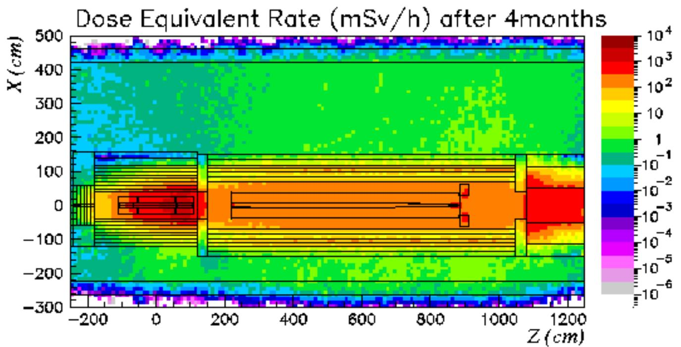
Figure 7 Total dose equivalent rate for cooling times of 2 months and 4 months for a longitudinal horizontal section at the level of the beam axis
