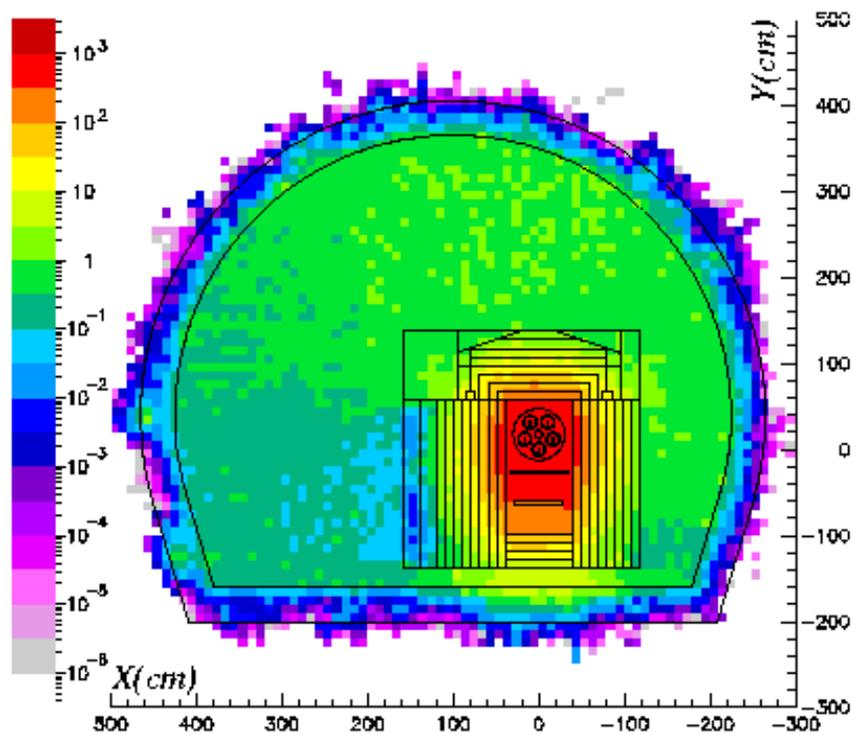
Figure 23 Total dose equivalent rate (mSv/h) after a cooling time of four months
