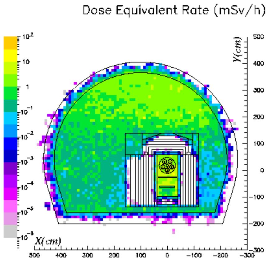
Figure 25 Horn area materials contribution after a cooling time of one week
