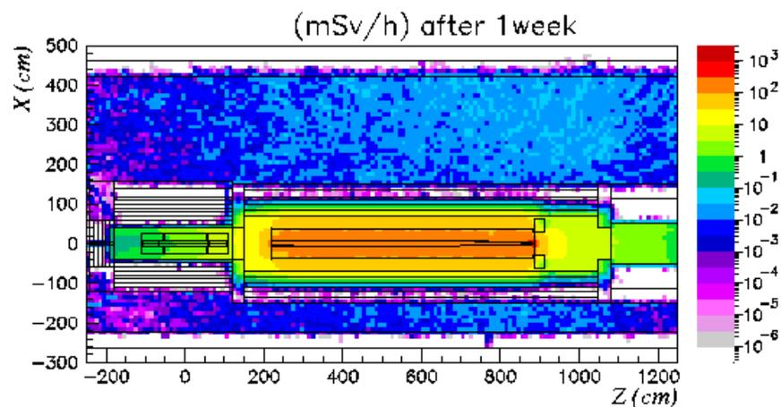
Figure 16 Dose equivalent rate from the horn tube material contribution
