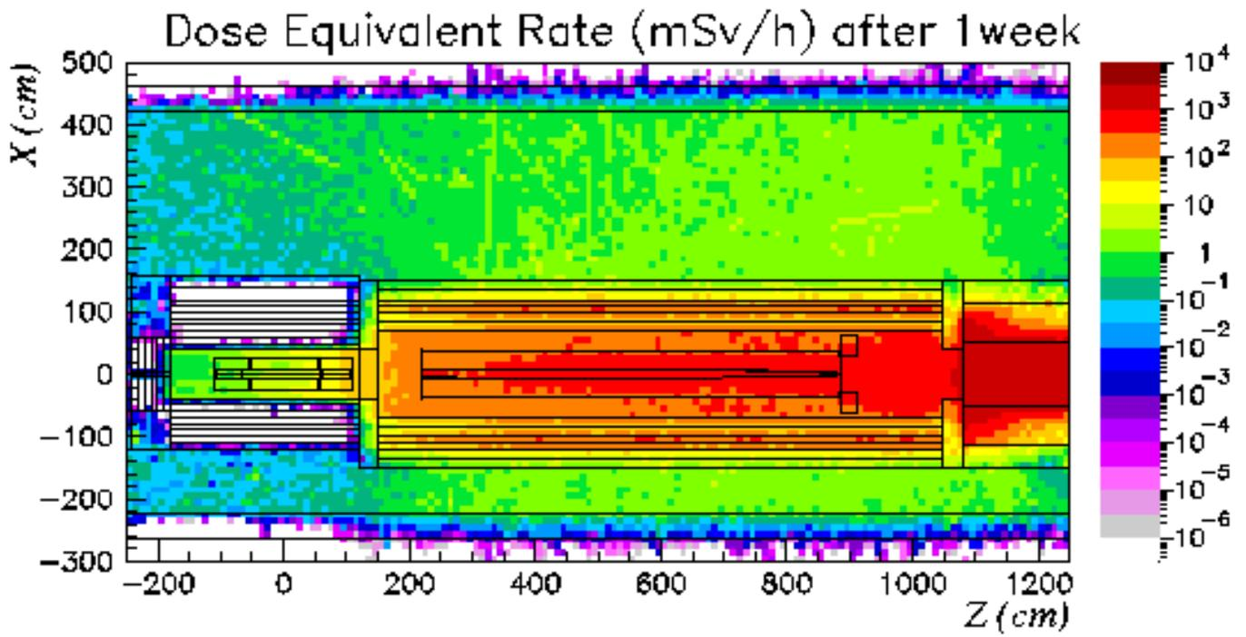
Figure 10 Contribution of the horn elements, horn shielding, electrical connections and collimator
