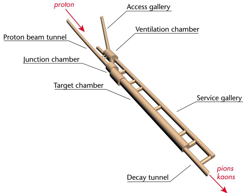
Figure 5: *The target chamber and its adjacent caverns and galleries: The service gallery will house power supplies, pumps and other equipment that must not be exposed to the high levels of radiation in the target region.*
