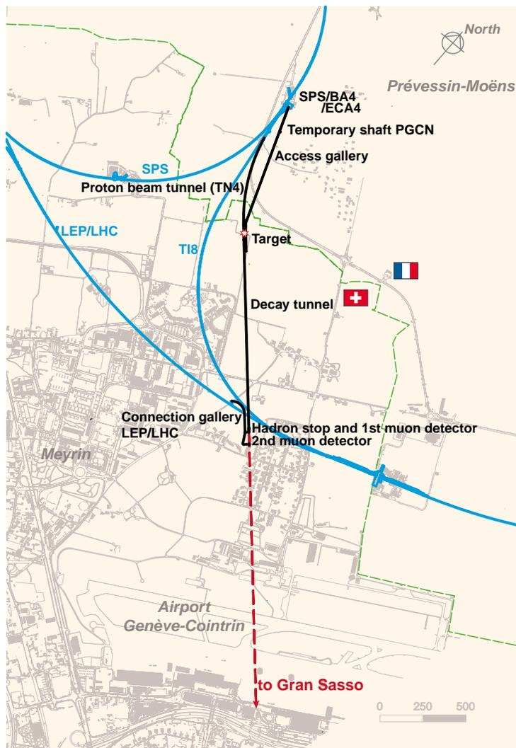
Figure 3: *The layout of the CNGS project at CERN, starting from the existing SPS accelerator at point 4. All the underground works will be conducted from the temporary shaft PGCN. No additional surface buildings will be needed for CNGS.*
