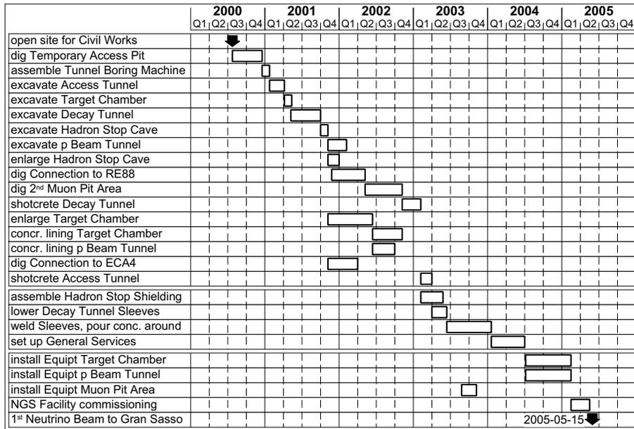
Figure 8: Construction schedule of the CNGS project.
