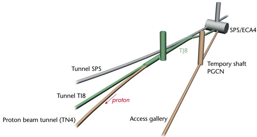
Figure 4: *The region around point 4 of the SPS: TI8 is the transfer tunnel from SPS to LHC, now under construction. The proton beam tunnel TN4 and the access gallery to the target chamber will be added for the CNGS project.*
