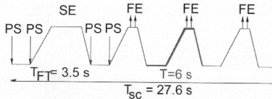
SPS operating for CNGS while filling LHC
