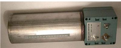
PS Booster Beam Loss Monitor Tests Confirmed that response time not an issue for CNGS (50ms between trains) More experiments and theoretical work required
