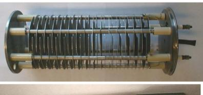
SPS Type Beam Loss Monitor Ionisation Chamber
