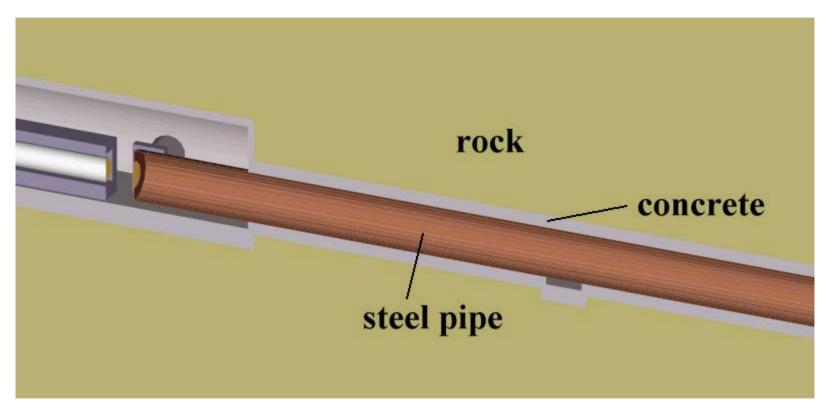
998 m long, evacuated 1-2 Torr2.45 m diameter18 mm thick
