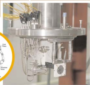
A prototype of the MINOS target. 4 \times 10^{14} protons, accelerated to 120 GeV, will strike the black graphite fins of the target every 1.9 seconds. Water cooling keeps the target from melting.
