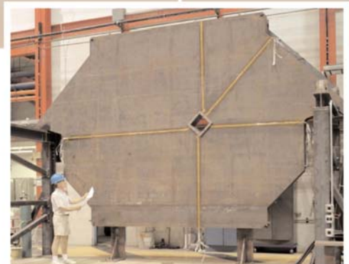
The near detector, located at Fermilab, is a smaller version of the main MINOS detector at Soudan, Minnesota. The near detector is used to verify the flavor of the neutrino beam at the source. The detector is smaller because the neutrino beam hasn't yet spread out very much.
