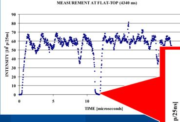
Measurements during the high intensity tests in 2004 → population in the gap ~1-2 %
