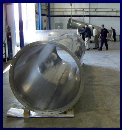
Length ~5m Diameter 800/1200mm 20 mbar over-pressure
