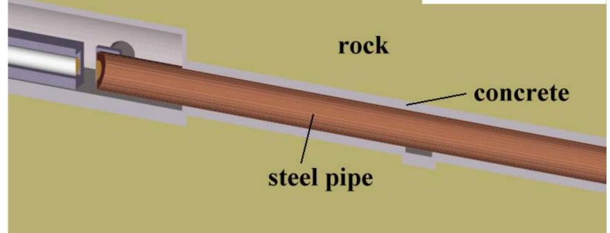
998 m long steel tube, surrounded by 50 cm of concrete evacuated to 1 Torr tube has 2.45 m diameter, is 18 mm thick
