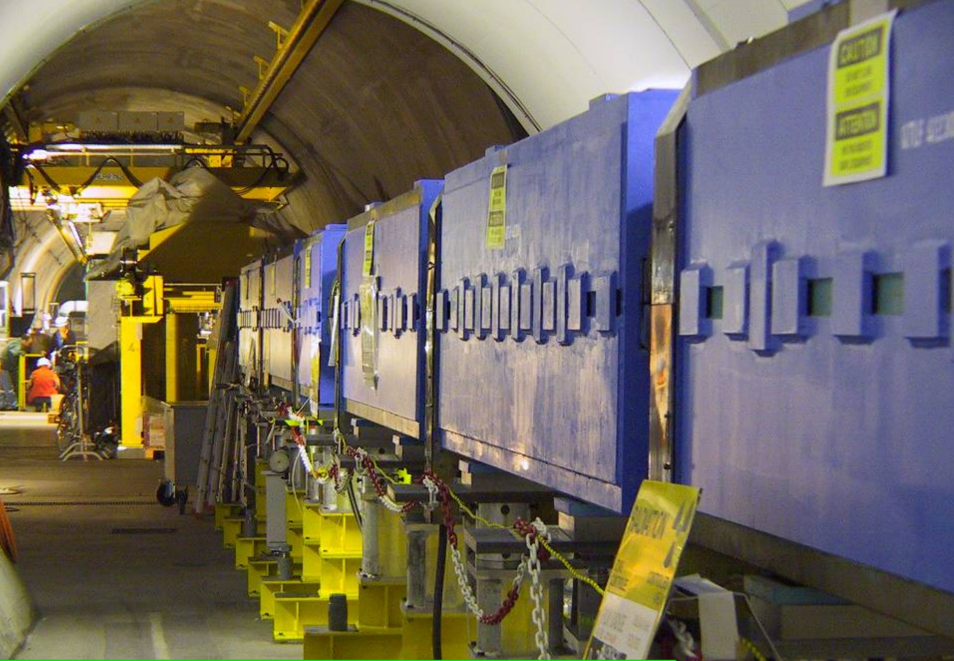
Final focusing onto the target (recuperated magnets)
