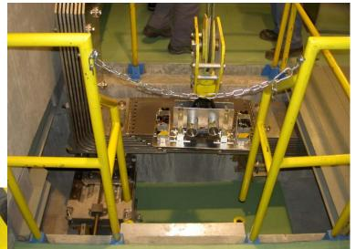
A survey platform has been developed to measure the residual dose rate in the CNGS cavern remotely
