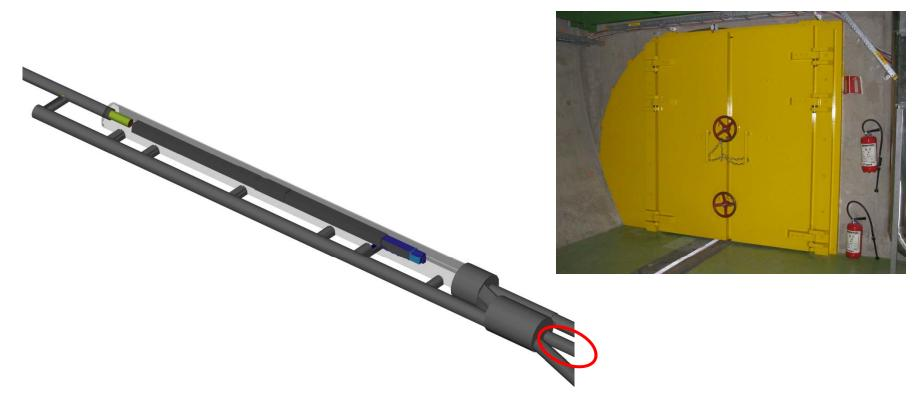
• A special stub tunnel has been constructed to serve as a radioactive storage area. Transport into the storage area can be made with a remote controlled transport vehicle. No need for long (time and distance) transports of radioactive components to a storage location somewhere on the surface.
