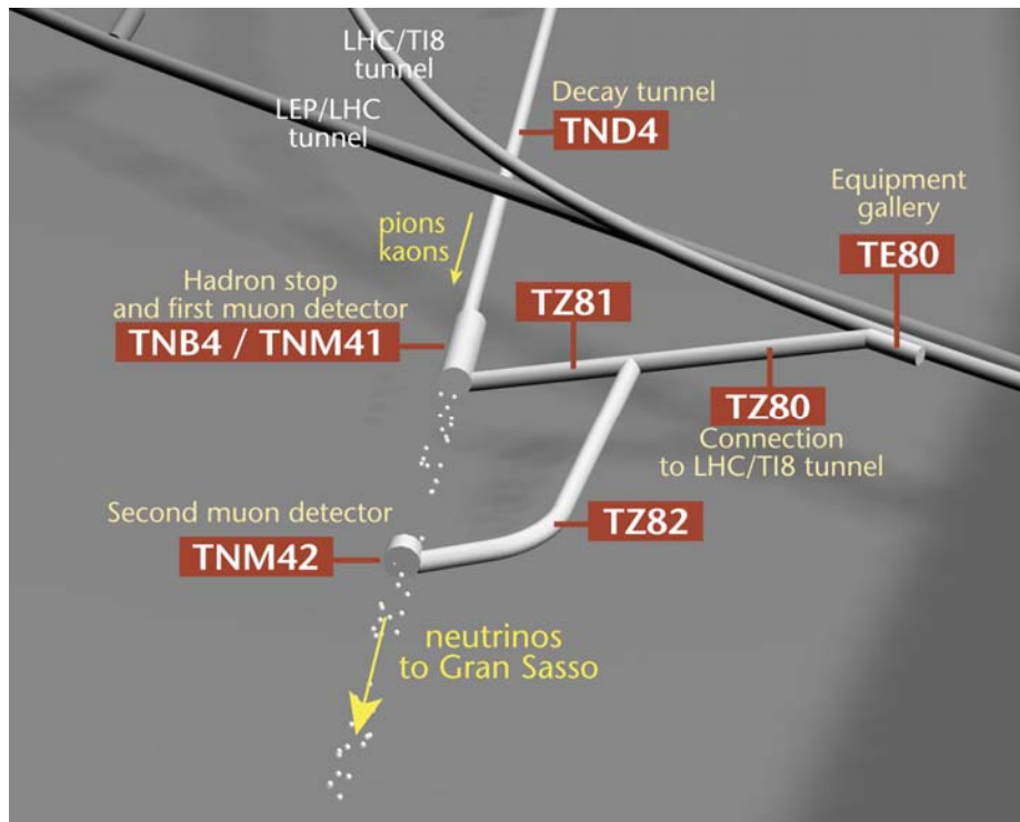
Figure 4: Hadron stop and muon chamber areas of CNGS
