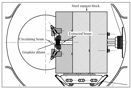
Figure 5: Cross section of the TPSG diluter.
