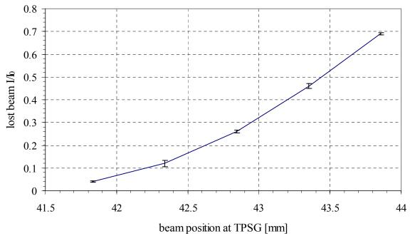
Figure 8: Relative losses at TPSG versus beam position.
