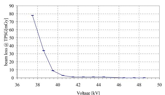
*Figure 9: Kicker voltage versus beam loss at TPSG.*
