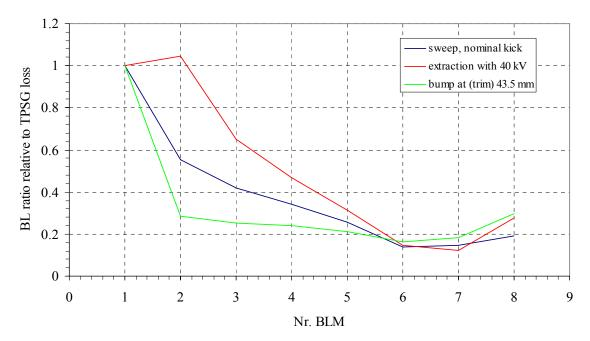
Figure 7: Comparison of loss patterns for losses on the inside, outside and swept across the TPSG.
