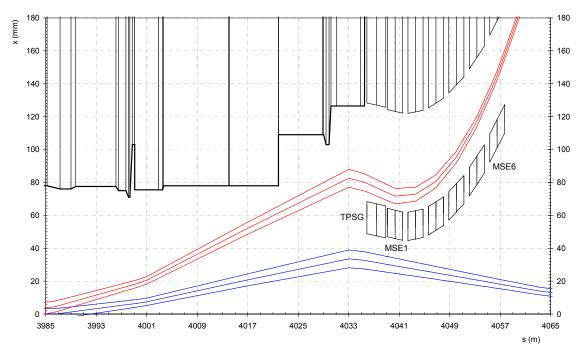
Figure 1 : Extraction region LSS4 with TPSG and septa and the circulating bumped orbit in blue and extracted trajectory in red.
