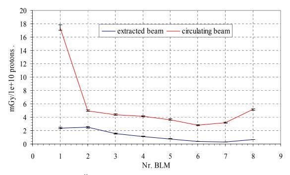
Figure 6: Beam loss per  $10^{10}$  protons for extracted (outside edge of TPSG) and circulating (inside edge of TPSG) beam.
