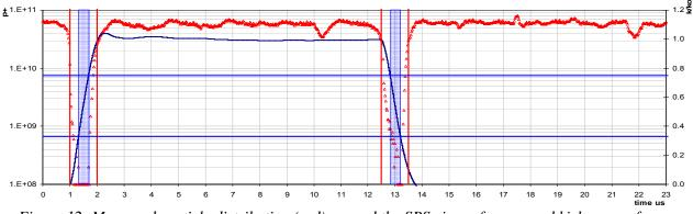
Figure 12: Measured particle distribution (red) around the SPS circumference and kicker waveform (dark blue) during first extraction.
