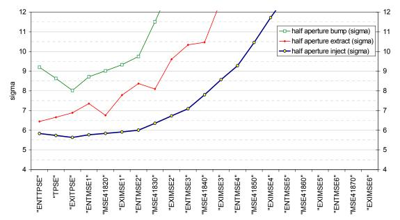
Figure 2: Calculated half aperture in the horizontal plane for the CNGS beam (14 – 400 GeV/c, 12  $\mu$ m emittance,  $\pm 1$  mm mechanical tolerance).
