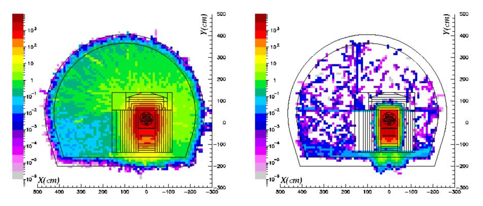
Figure 27 Target shielding contribution after a cooling time of one week
