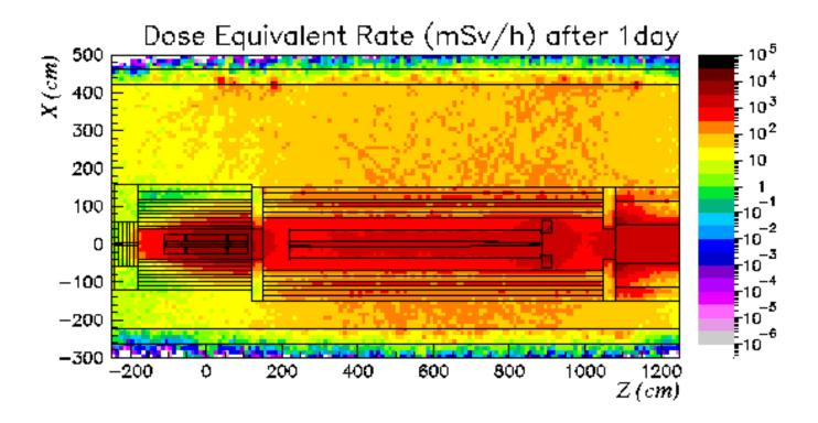
Figure 5 Total dose equivalent rate for a cooling time of 1 day for a longitudinal horizontal section at the level of the beam axis
