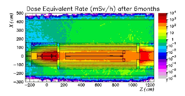
Figure 8 Total dose equivalent rate for a cooling time of 6 months for a longitudinal horizontal section at the level of the beam axis
