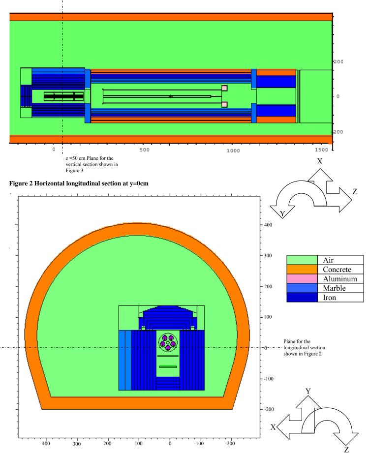
Figure 3 Vertical transverse section at z=50cm (center of the target unit)
