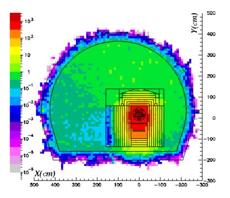
Figure 24 Total dose equivalent rate (mSv/h) after a cooling time of six months
