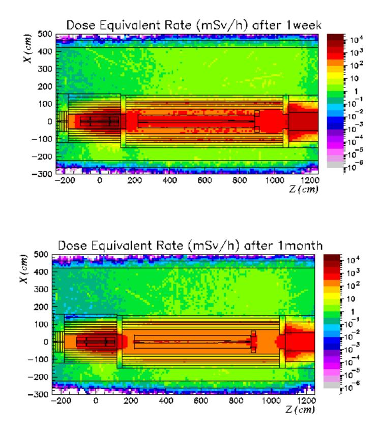
Figure 6 Total dose equivalent rate for cooling times of 1 week and 1 month for a longitudinal horizontal section at the level of the beam axis
