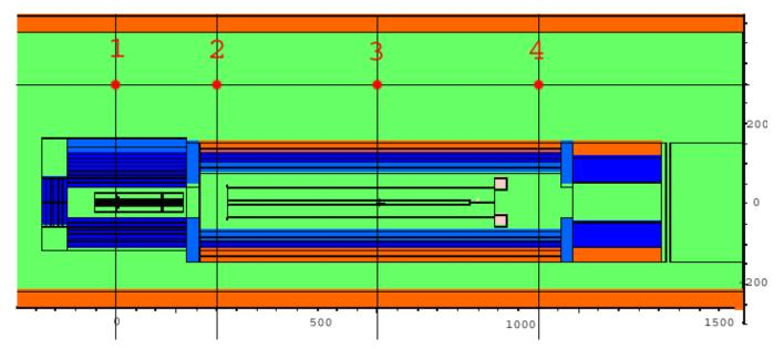
Figure 14 Horizontal longitudinal section at y=0 cm showing the locations for which dose equivalent rates are given in table 3
