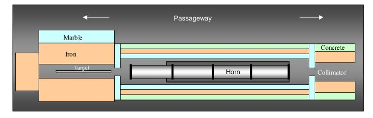
Figure 1 Schematic view of the target and horn area
