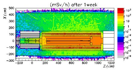
Figure 15 Dose equivalent rate from the horn shielding contribution
