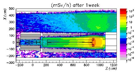
Figure 17 Dose equivalent rate from the stripline and elements of the shielding opening contribution
