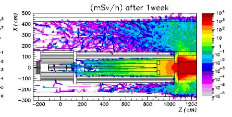
Figure 18 Dose equivalent rate of the collimator contribution
