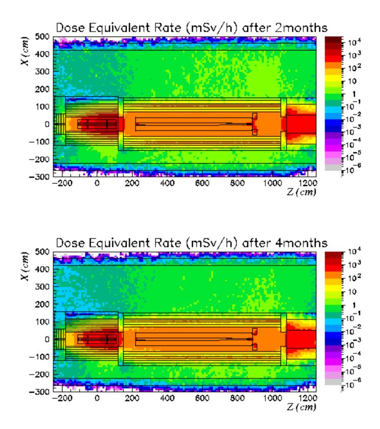
Figure 7 Total dose equivalent rate for cooling times of 2 months and 4 months for a longitudinal horizontal section at the level of the beam axis
