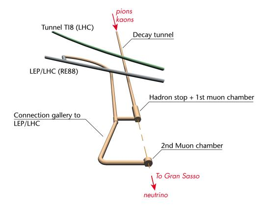
Figure 6: The region of the CNGS beam dump (hadron stop): the exisiting LHC tunnel and the TI8 transfer line are passing above the CNGS decay tunnel. Access to the muon detectors is via the LHC tunnel.
