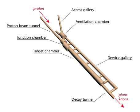
Figure 5: The target chamber and its adjacent caverns and galleries: The service gallery will house power supplies, pumps and other equipment that must not be exposed to the high levels of radiation in the target region.
