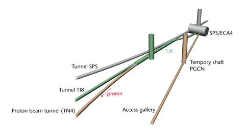
Figure 4: The region around point 4 of the SPS: TI8 is the transfer tunnel from SPS to LHC, now under construction. The proton beam tunnel TN4 and the access gallery to the target chamber will be added for the CNGS project.
