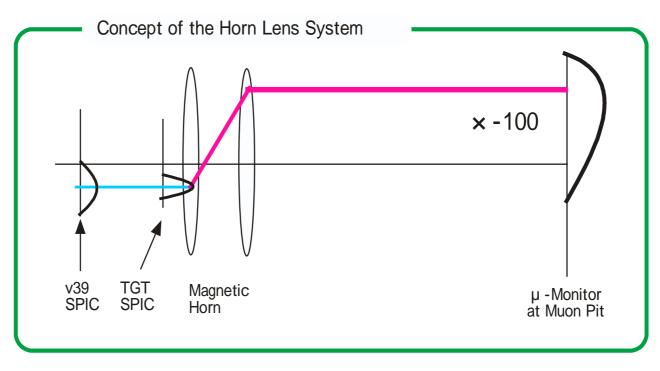
The Horn functions as a lens with the Magnification of  $\sim$  -100.
