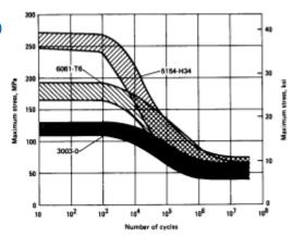
The fatigue life of welded joints at high loads varies with the alloy. As the load is decreased, differences disappear until, at about one to ten million cycles of axial loading (R = 0), the fatigue strength of an arc-welded joint is approximately the same regardless of alloy and is 50 to 70% that of the unwelded alloy. Typical data are given in the above graph for three aluminum alloys. Specimens were from 9.5-mm ( $\frac{1}{2}$ -in.) plate; weld reinforcement removed; axial loading; R = 0.
