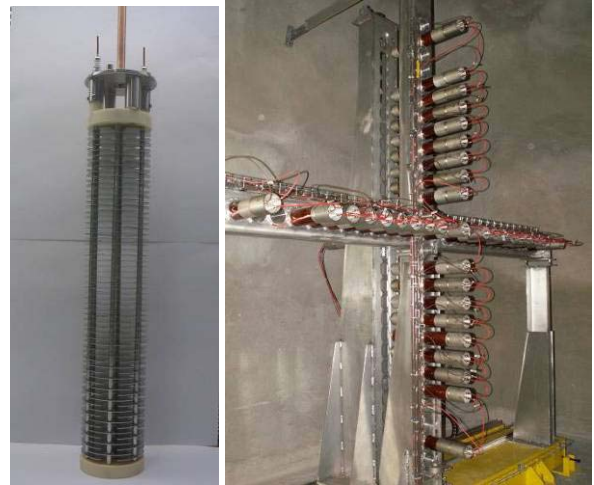
Figure 4: Left: a single muon detector, without its stainless steel casing. Right: A muon detector station with the muon detectors arranged in a cross-shaped array.
