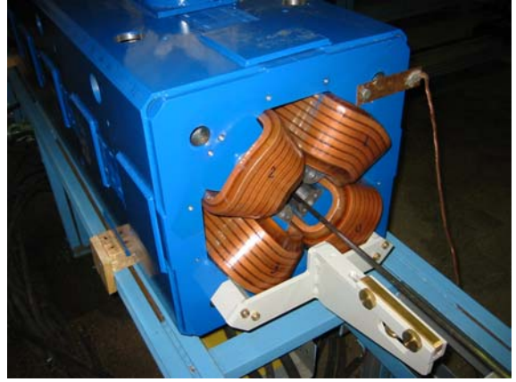
Fig.4. First QTG magnet on the magnetic measurement bench at BINP.
